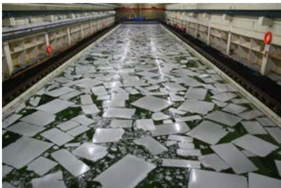
Figure 5: Managed Ice in a model test basin
