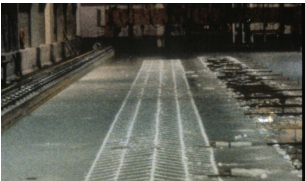
Figure 3: Cutting pattern of pre-sawn ice
