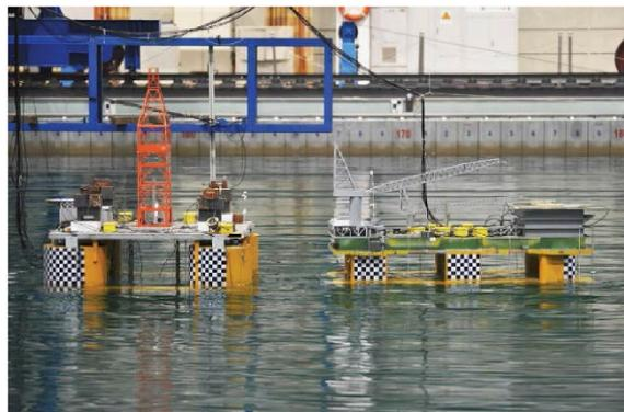
Figure 18: Experiment of TLP-TAD coupled system (Dong et al., 2019)
