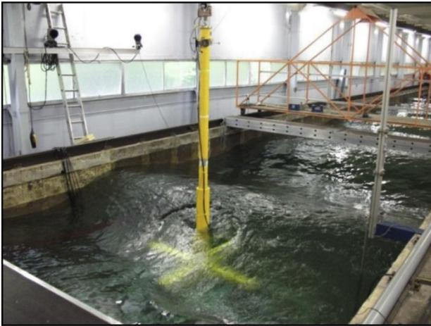
Figure 24: Extreme irregular wave test (Oguz et al., 2018)
