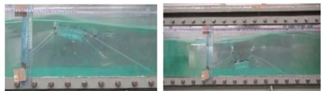
Figure 62: Controllable depth cage model test when the cage was at water surface (left) and at the submerged depth (right) (Yu et al., 2018)
