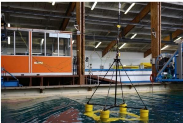
Figure 89: Scale model during wave tank tests (Matoug et al., 2020)
