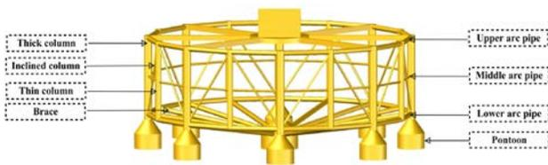
Figure 63: Primary frame of the fish farm (Zhao et al., 2019)
