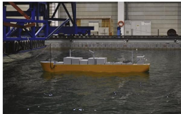
Figure 20: FLNG vessel model test setup in the basin (Z.-Q. Hu et al., 2017)
