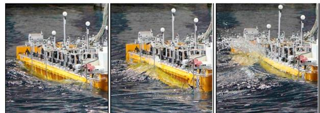
Figure 3: Evolution of a beam sea extreme green water event during model tests (Silva et al., 2017a)
