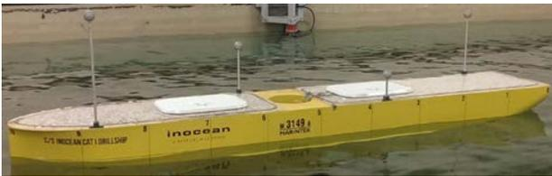
Figure 28: The model test for thruster-assisted position mooring (Bjørnø et al., 2017)
