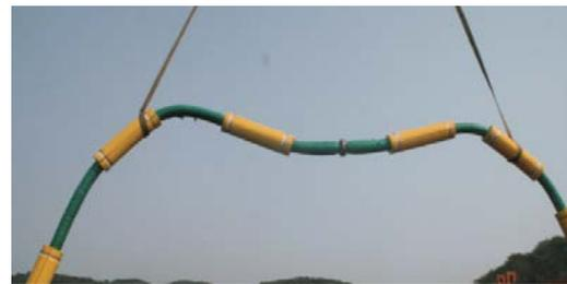
Figure 135: Flexible hoses with buoyancy materials (Yoon et al., 2011)
