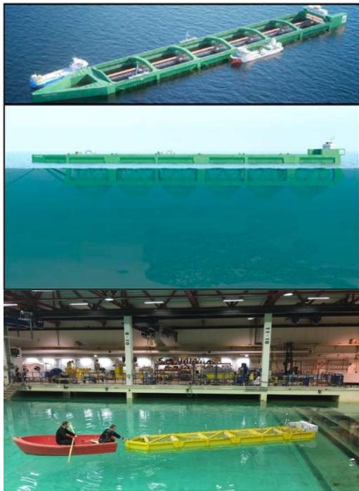
Figure 48: Havfarm. (a) concept (<https://www.nskshipdesign.com/designs/aquaculture/fishfarm-2/fish-farm/>) (b) Model tests (Picture courtesy of SINTEF Ocean).
