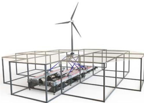
Figure 77: 6-DoF Robotic platform “HexaFloat” for wind tunnel tests (Bayati et al., 2014)
