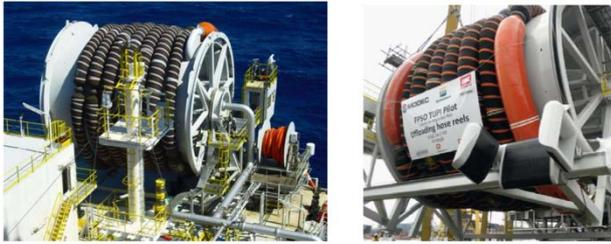
Figure 139: Spooled riser applied on a vessel (Rhee et al., 2013)
