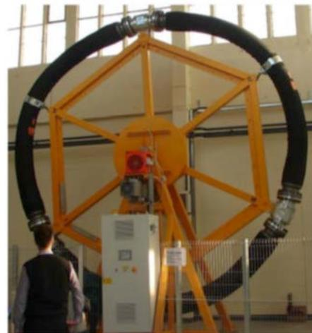
Figure 145: Rotating full-scale abrasion tester (Neale et al., 2017)
