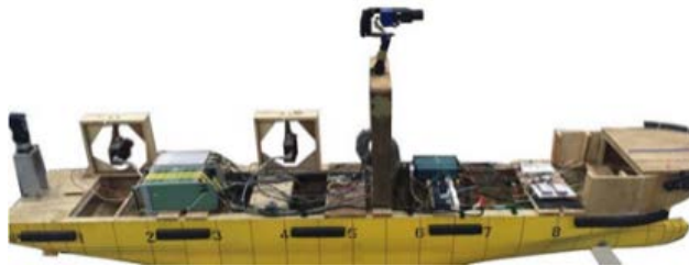
Ship model with active pitch oscillating bow fin (Chiu et al., 2018)
