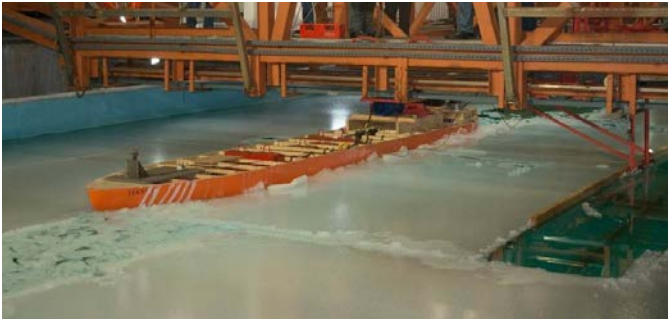
Towing tests of ship in compressive ice (KSRC)
