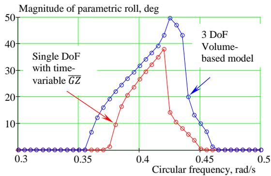
Figure 27: Magnitude of parametric roll. Weather-tight volume is included
