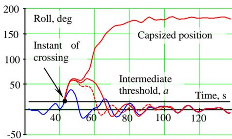
Figure 22: Motion perturbation for computing the capsizing metric
