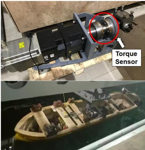
Figure 24: Forced roll mechanism developed by MARIC
