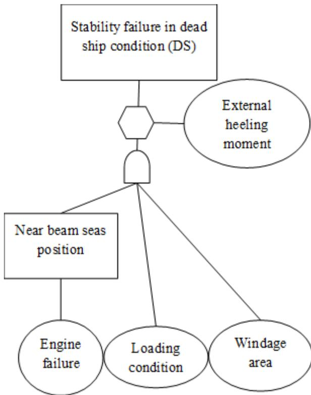
Figure 15: Fault tree for stability failure on dead ship condition (DS)
