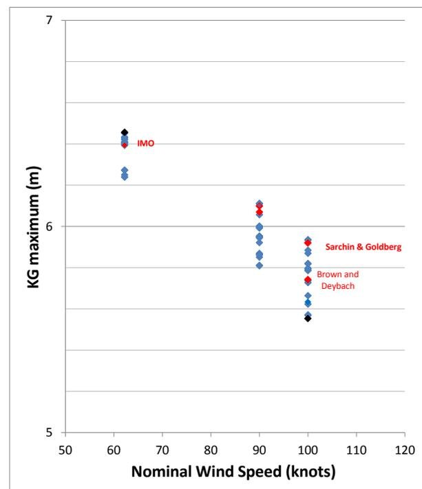
Figure 9:  $KG_{max}$  due to wind for a set of rules
