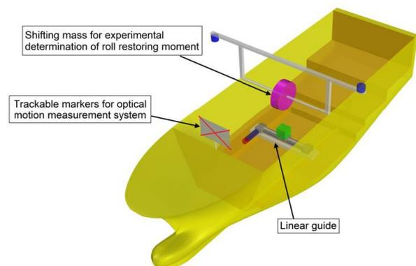
Figure 23: Moving mass type RMGs (Up: Park et al., 2018; Down: Oliva-Remola, 2018)
