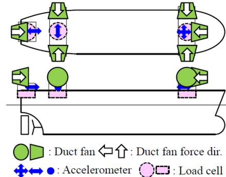
Figure 4: Configuration of onboard part of the wind loads simulator.
