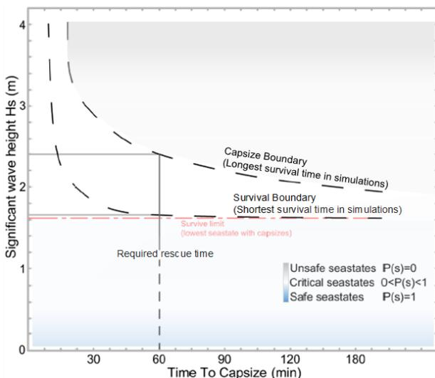
Figure 31: Capsize and survival boundary concept with indication of the safe and unsafe regions with respect to change of the Time to Capsize as a function of the significant wave height. (Atzampos, 2019)
