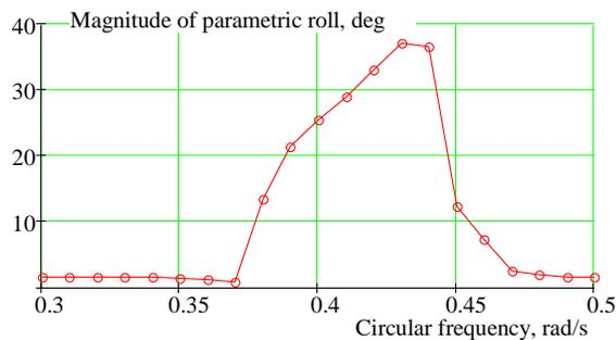
Figure 28: Magnitude of parametric roll computed with LAMP-2 (Shin et al. 2004)
