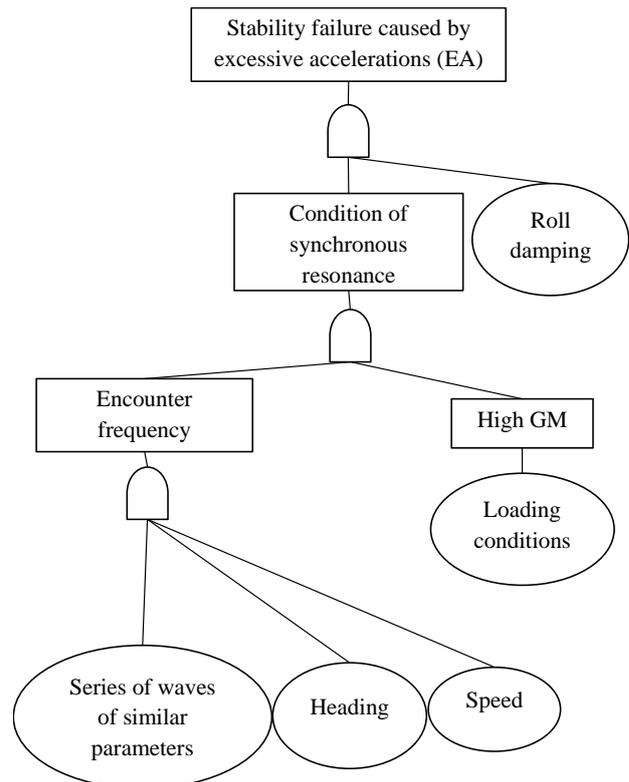
Figure 16: Fault tree for stability failure on excessive acceleration (EA)
