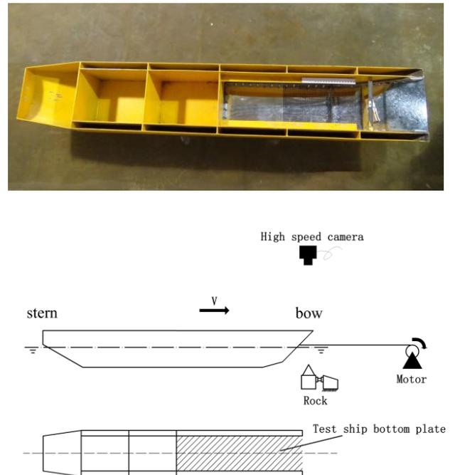
Figure 1: Experimental set-up for grounding from Zhu et al. (2018)
