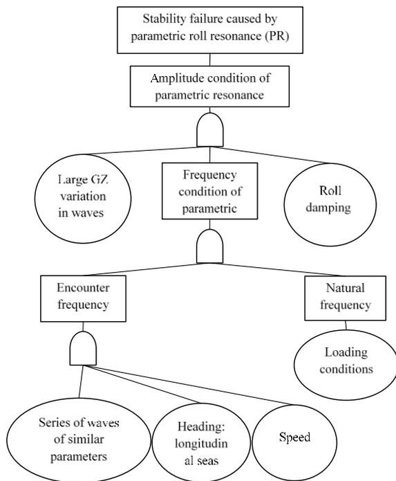
Figure 13: Fault tree for stability failure caused by parametric roll (PR)
