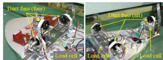
Figure 5: Wind loads simulator on a model ship
