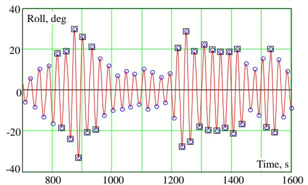
Figure 29: Data acquisition for SSD: mean-crossing peaks (circles), 1/3<sup>rd</sup> largest peaks (squares)
