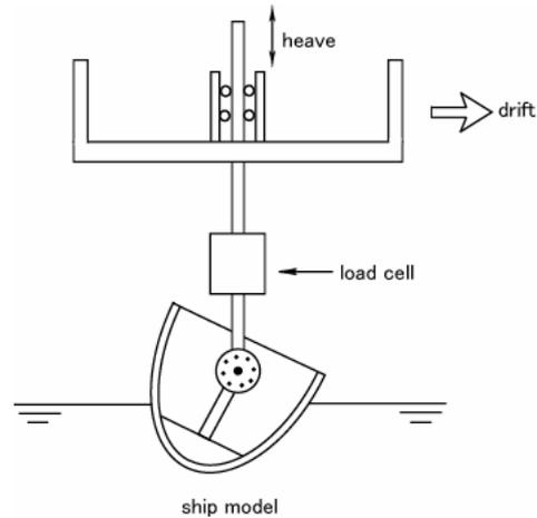
Figure 7: Set up proposed by IMO for hydrodynamic forces estimation due to current
