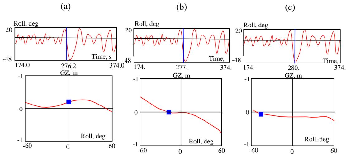
Figure 10: Time history and evolution of  $\overline{GZ}$  curve in irregular waves a) zero roll angle; b) zero stiffness; c) Roll angle excursion
