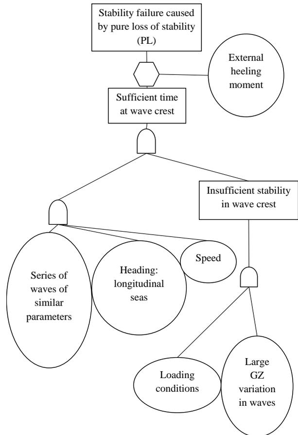
Figure 14: Fault tree for stability failure caused by pure loss of stability (PL)
