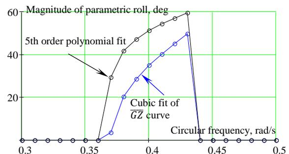
Figure 25: Magnitude of parametric roll as a function of the wave frequency
