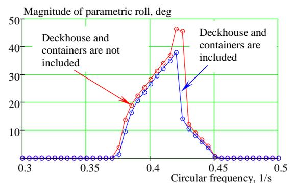
Figure 26: Magnitude of parametric roll by numerical integration of 1-DoF roll equation
