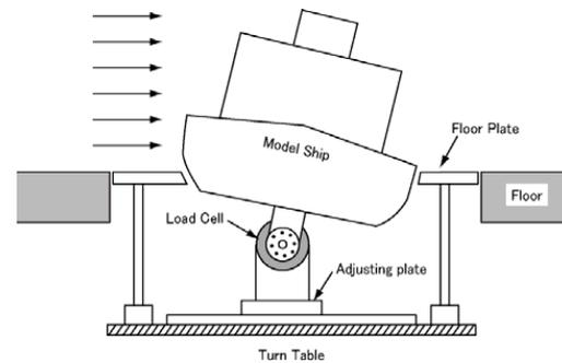
Figure 8: set up proposed by IMO for aerodynamic forces estimation
