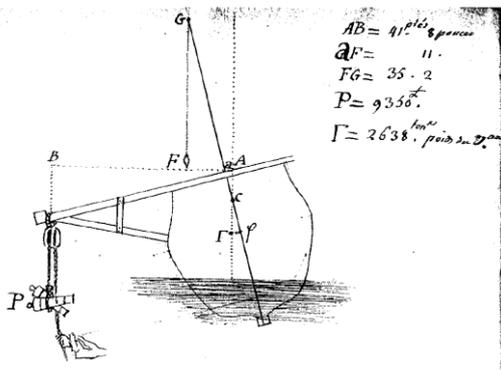
Figure 32: First referenced inclining experiment in 1748, according Nowacki and Ferreiro (2003)
