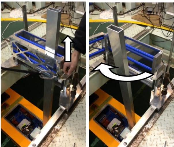
Figure 3. Opening mechanism of apparatus
