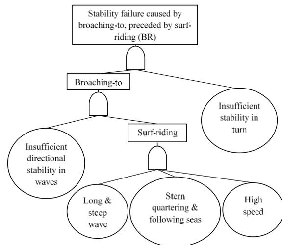
Figure 12: Fault tree for stability failure caused by broaching-to (BR)
