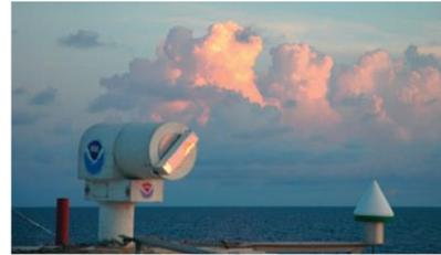
Figure 60 Doppler LIDAR scanner on a vessel [Pichugina, 2012]
