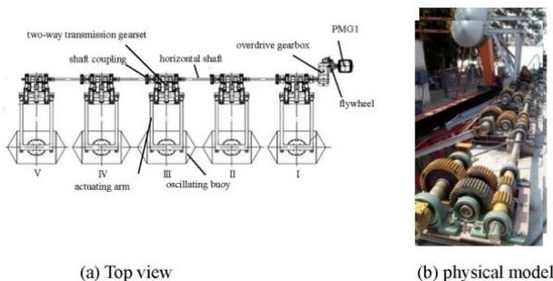
Figure 15: Array drive mode from Yang et al., 2019.
