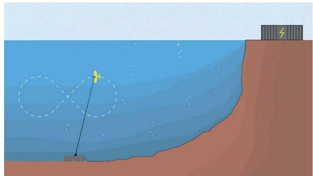
Figure 9: The orbital path of Deep Green device, Miesto (2021) turbine.
