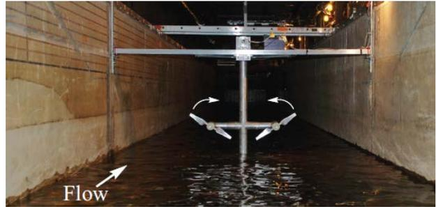
Figure 3: A 1:40 scale dual rotor horizontal-axis current turbine (DOE-RM1) channel facility (from Hill et al. (2020))
