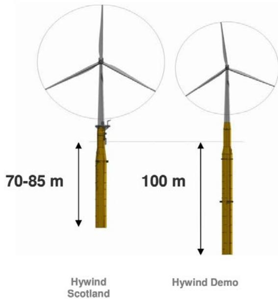
Figure 11: Hywind Scotland (2017) and Hywind Demo (2009) Spar floating offshore wind turbines (xodus group, 2013).
