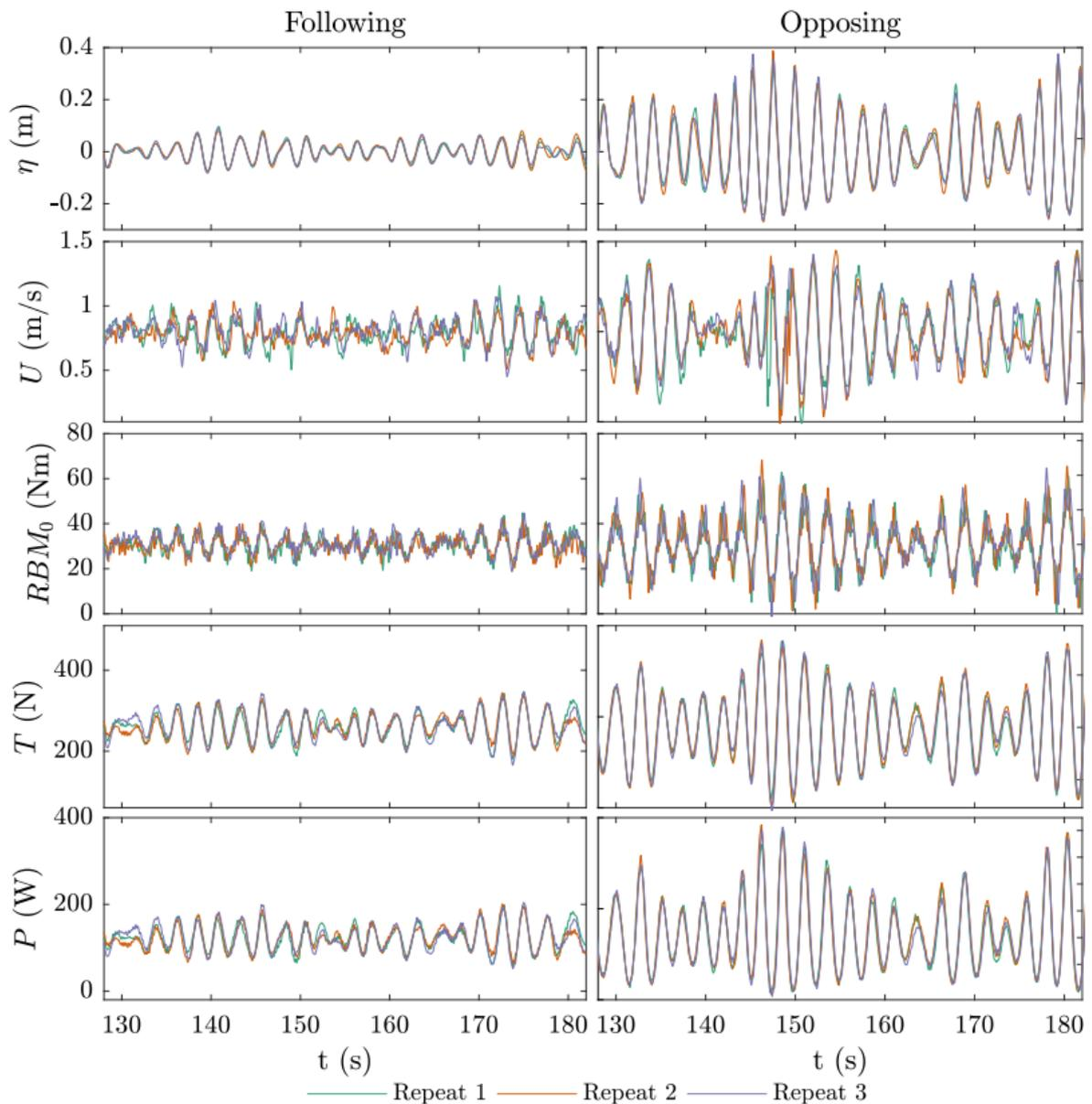
Figure 18: Time-domain results of key environmental and turbine parameters for the opposing and following wave conditions. The three repeats of each conditions are shown for each parameter;  $H$  is the surface elevation;  $U$  is the streamwise velocity, 0.4 m beneath the surface;  $RBM_0$  is streamwise blade root bending moment sensors;  $T$  is rotor-based thrust measurement;  $P$  is rotor power.
