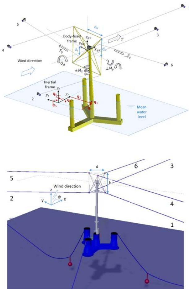
Figure 22: Real-Time Hybrid Model (ReaTHM) testing setup with cable driven parallel robots: NOWITECH (top); LIFES50+ (bottom). From Chabaud et al. 2018.
