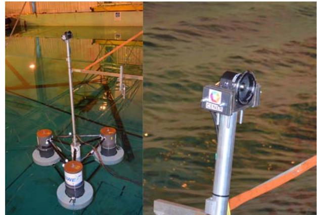
Figure 21: Hybrid testing with a single ducted fan used in the EU INNWIND-project (courtesy of CENER).
