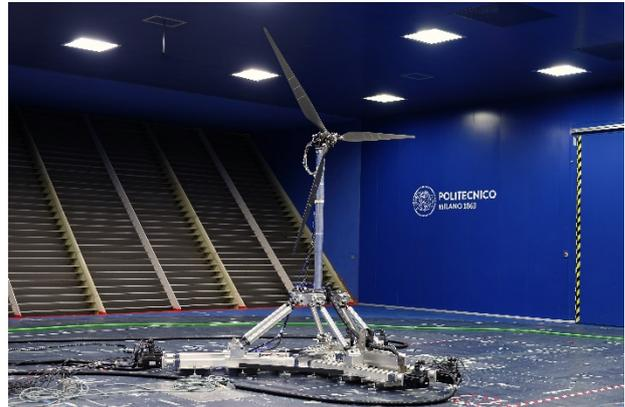
Figure 25: 6DOF hybrid setup of a floating wind turbine in a wind tunnel (from Belloli et al., 2020; courtesy of Politecnico di Milano).
