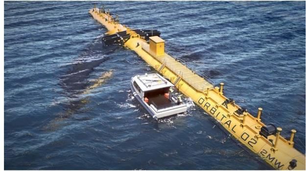
Figure 8: Orbital marine power twin 2MW device. (Orbital marine power, 2021)
