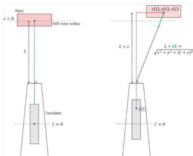
Figure 14: Relative displacement of the floater with respect to the PTO from Giassi et al., 2020.
