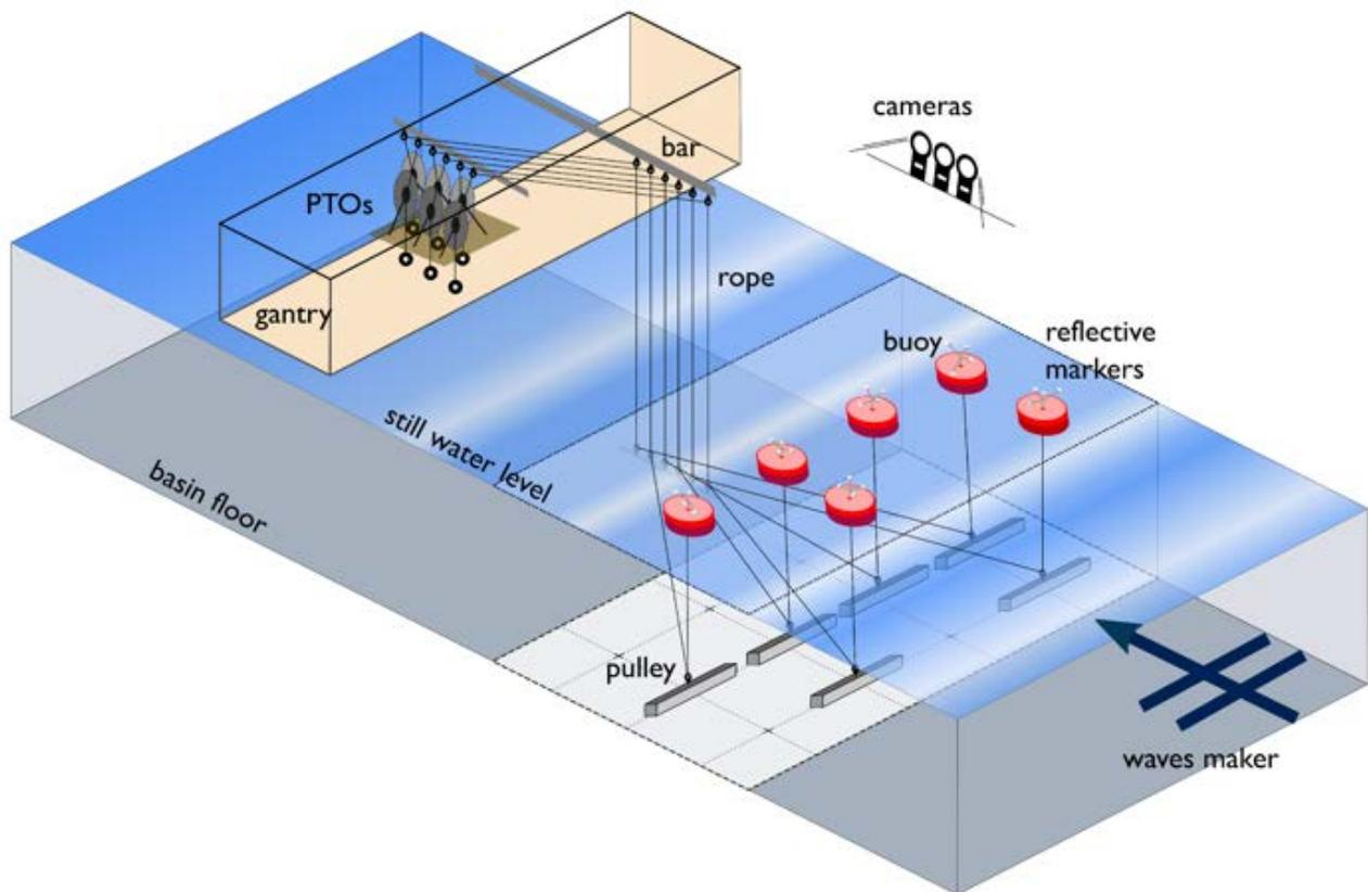
Figure 13: Layout of the array with each WEC moving in 6DOF (from Giassi et al., 2020)
