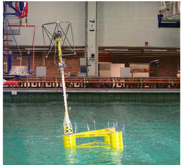
Figure 23: Real-Time Hybrid Model (ReaTHM) tests of the INO WINDMOOR 12MW FOWT (courtesy of SINTEF Ocean).
