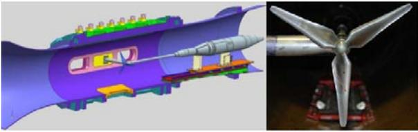
Figure 2: A 1:8.7 scale horizontal-axis current turbine (DOE-MHKF1) in cavitation tunnel (from Fontaine et al. (2013))
