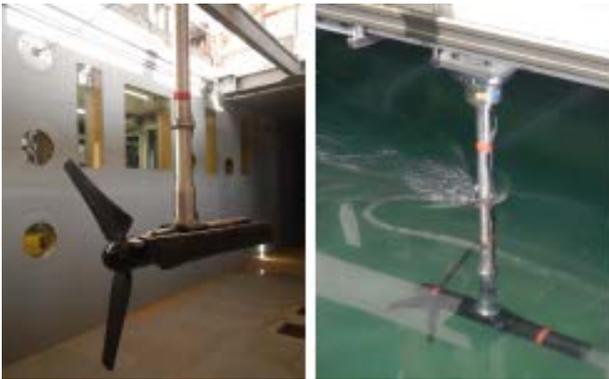
Figure 1: Three-bladed “round-robin” horizontal instrumented turbine in water flume and tow tank (From Gaurier et al. (2015))
