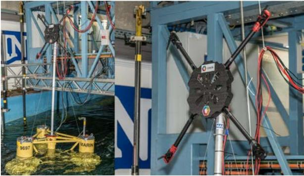
Figure 24: MARINET2 tests with CENER's multi-fan actuator system tested at MARIN (courtesy of CENER).
