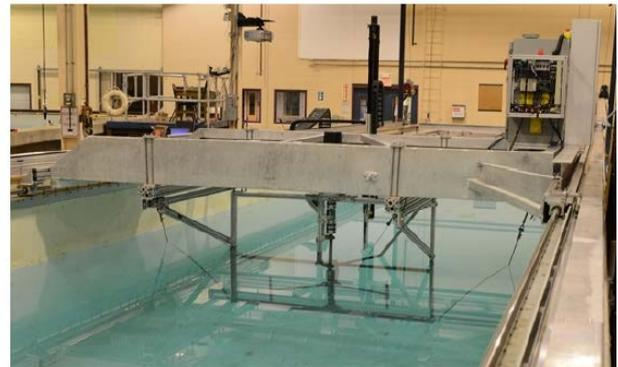
Figure 4: A 1:6 scale cross-flow turbine (DOE-RM2) setup up in tow tank (from Wosnik et al. (2015))
