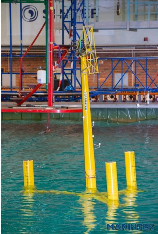
Figure 5: NOWITECH model test of a 5MW FWT (courtesy of SINTEF Ocean).
