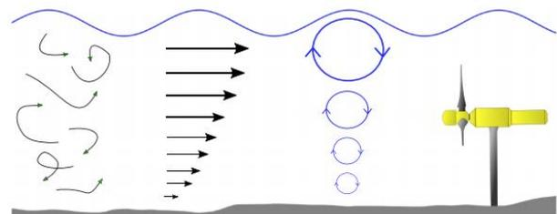
Figure 17: Diagram of the key causes of unsteady loads on tidal turbines (Draycott et al. 2019).
