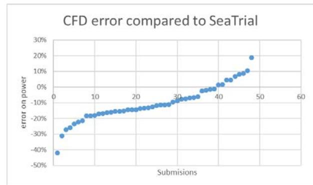
Figure 9. CFD error of predicted power for a given speed compared to sea trial result.
