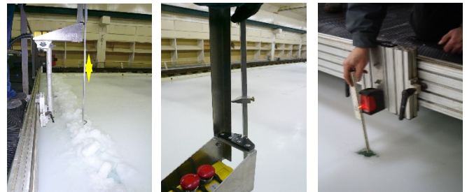
Figure 15 Ridge-profiling device to determine keel depth and sail height
