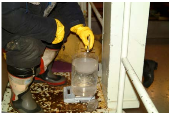
Figure 8: Force balance measurement without displacement recording (Option C)
