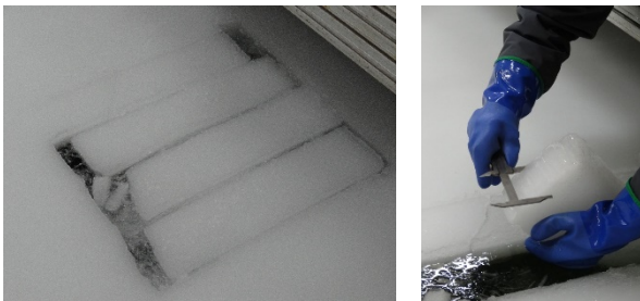
Figure 14: Ice thickness measurements with calliper
