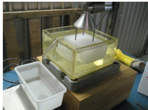
Figure 6: Ex-situ density measurement setup (Option A)
