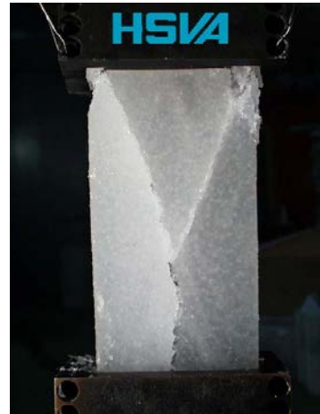
Figure 11: Compressive ex-situ test setup
