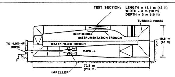
Approx. length of water circuit measured around the centerlines = 152 m (532 ft)
