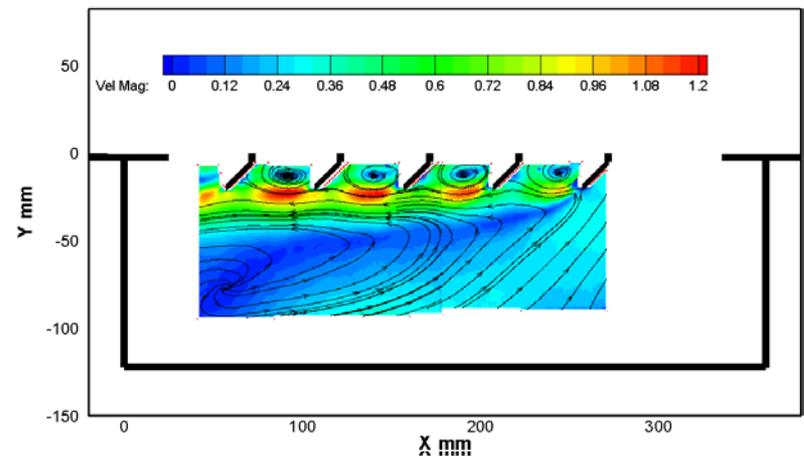
Flow inside a cavity with 45° block
