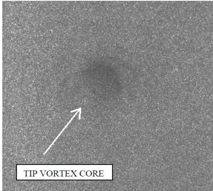
Example of an otherwise optimal seeding which is negatively affected by the high shear region inside a vortex core
