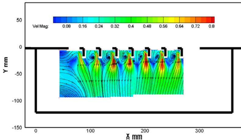
Flow inside a cavity with straight block
