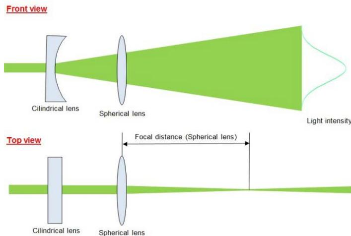
A typical light-sheet optics arrangement
