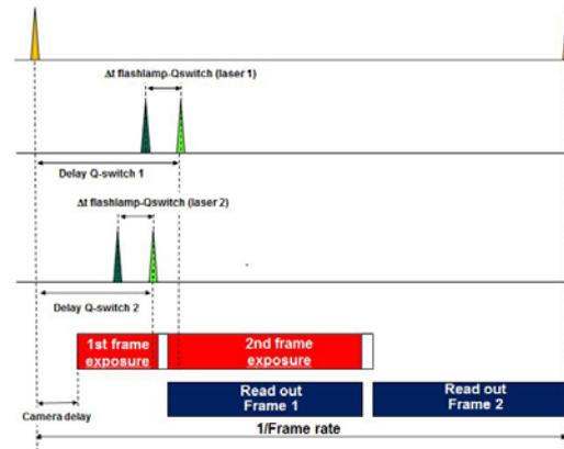
A typical PIV timing diagram
