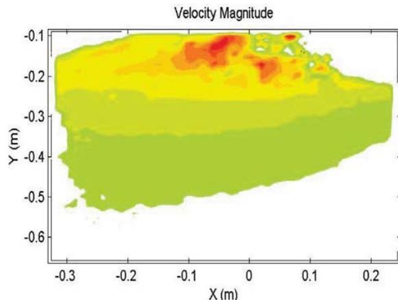
PIV measurement of near-surface velocity field in breaking wave.
