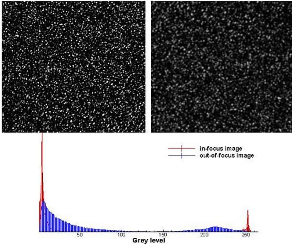
Adjustment of the camera focus by the examination of the grey level distribution
