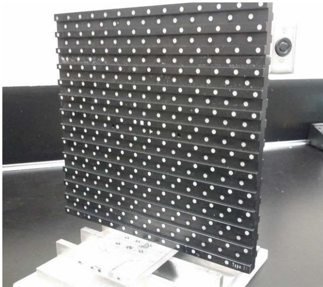
A double-plane-double-side type SPIV calibration target
