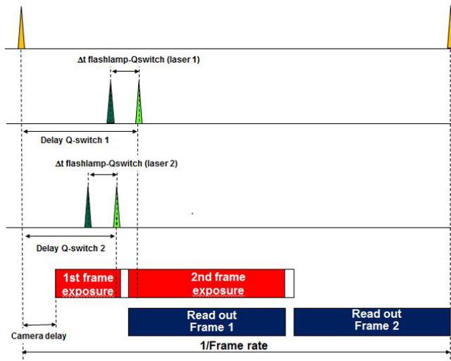
A typical PIV timing diagram
