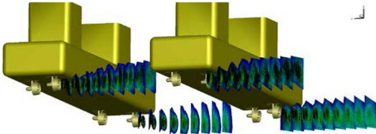
Figure 7.3.3 Measured Wake Velocity Field
