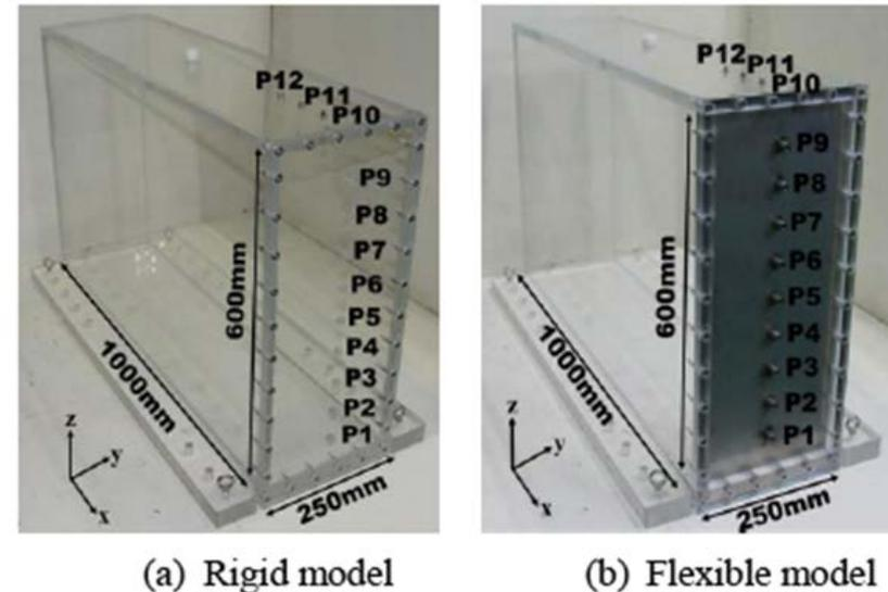
Figure 2.3.2.3 Rigid and Flexible Models and Locations of Pressure Transducers (Choi et al., 2012)
