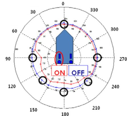
Thrust Loss due to Thruster-Thruster Interaction (Song et al., 2013 )
