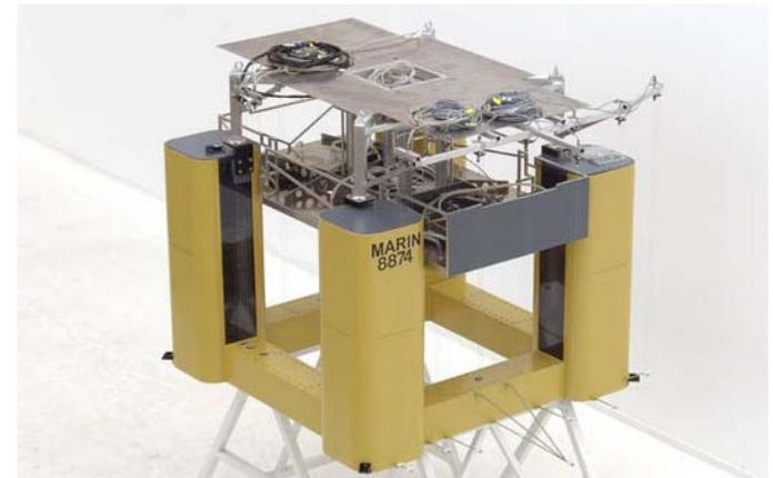
Figure 2.1.2.1 The TLP Model Used in CresT (Hennig et al., 2011)
