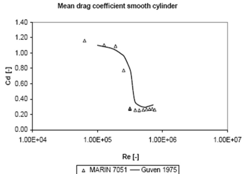
Figure 5.1.3 Drag Coefficient for Smooth Cylinder – Experimental
