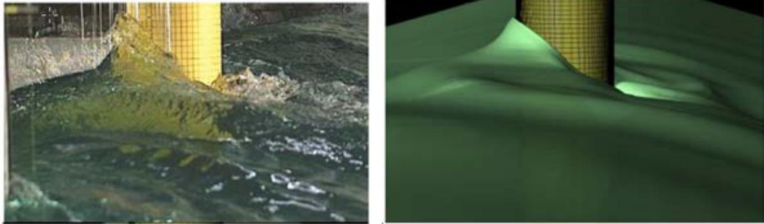
Figure 6.5.1 Experimental Wave Profiles (Stansberg and Kristiansen, 2005) and Numerical Predictions for the Case of  $T=15s$ ,  $H=35m$  (Yoon et al., 2013)
