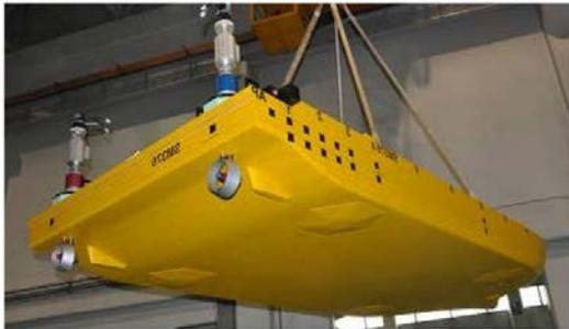
Ship Model for Thruster-Thruster/Hull Interaction Tests
