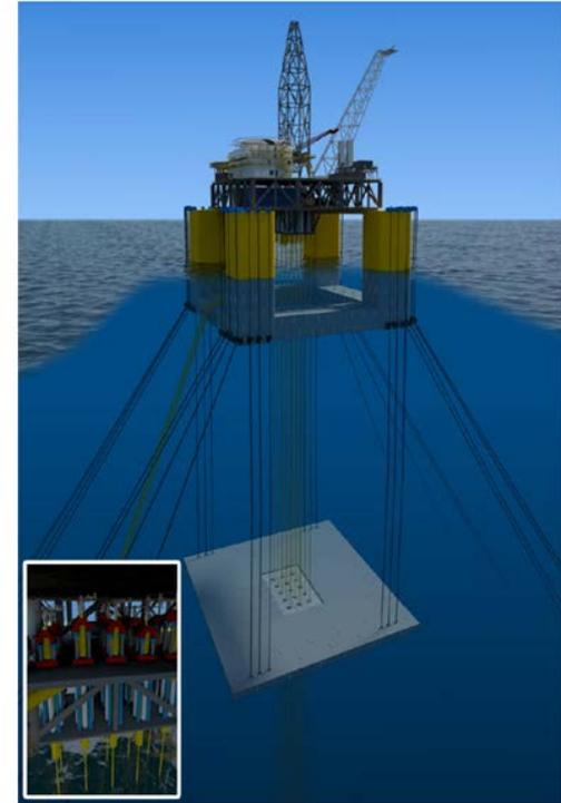
Figure 2.1.3.1 The Free Hanging Solid Ballast (FHSB) Semi (Mansour and Kumar, 2013)
