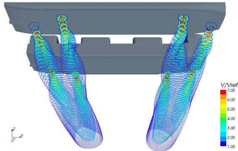
Figure 7.2.5 Downwash of Active Thrusters, Azimuth 270 deg (Ottens et al., 2011)
