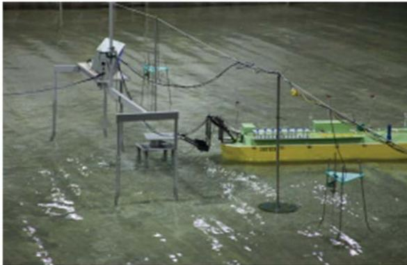
Figure 9.1 Tower Yoke Mooring System (Kim et al., 2011 )
