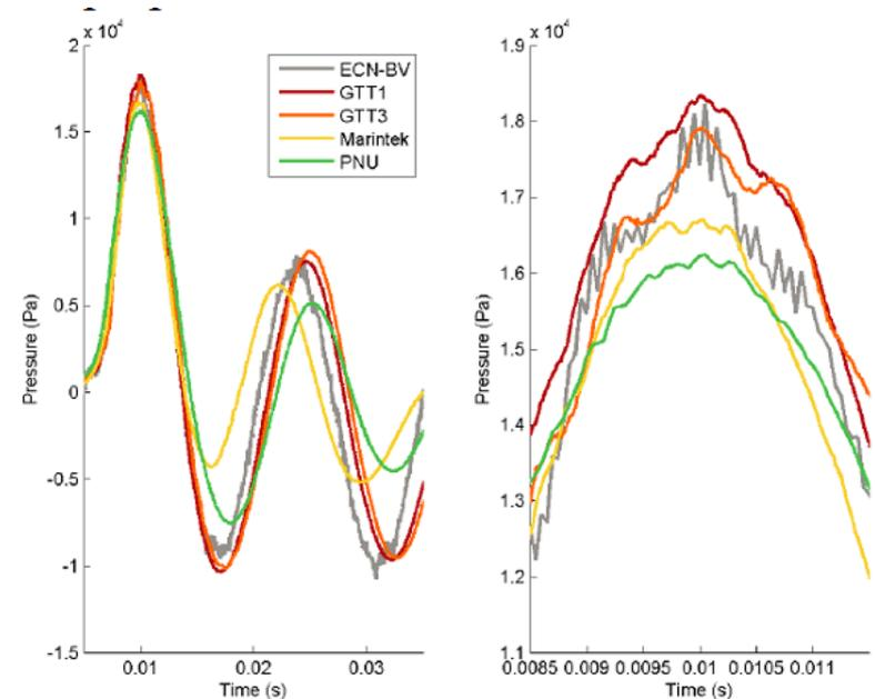
Figure 2.3.2.1: Representative Pressure Time Histories by Six Participants for A Single Impact Wave (Loysel et al., 2013)
