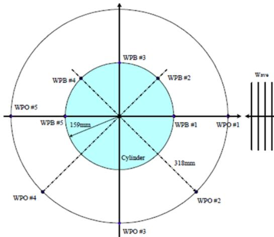
Placement of Wave Probe on and around the Cylinder
