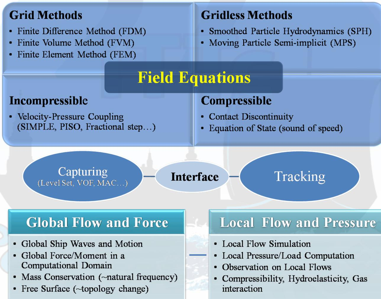
Overall status of the art of CFD schemes for free surface flow: Field equation solvers
