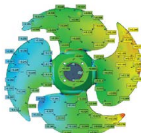
Optical scan on a CP propeller (deviation from its theoretical geometry, pressure side –suction side) (Dang et al., 2012)
