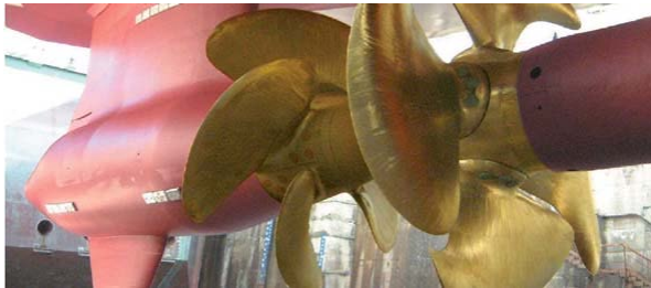
The main propeller (right) with counter rotating, 360 degree azimuthing, ABB Azipod thruster on 200 TEU Container Feeder vessel (Henderson, 2013)
