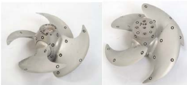
Optical scan on a CP propeller (deviation from its theoretical geometry, pressure side –suction side) (Dang et al., 2012)
