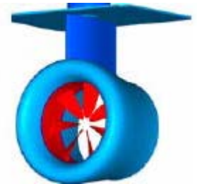
Rim-Driven Hubless Composite Props (Büchler and Erdman, 2006)
