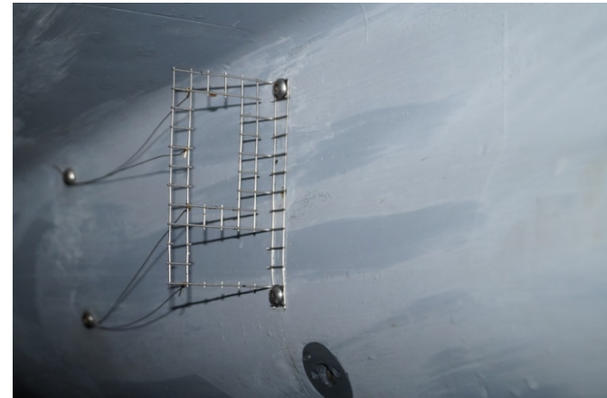
Dummy model, optimized on the base of an adjoint sensitivity analysis
