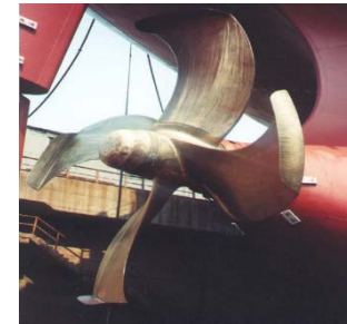
Backward tip rake propeller (Sistemar) Sanchez-Caja et al. (2012) ; Inuakai (2013)
