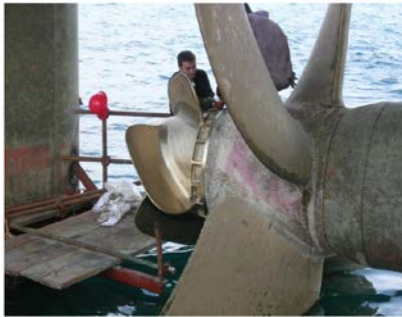
PBCF to a full scale ship (Hansen et al. , 2011)
