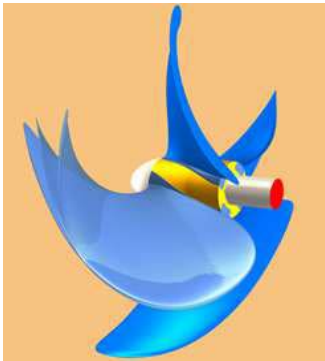
Elastic blade deformation on a composite propeller (Young, 2012)
