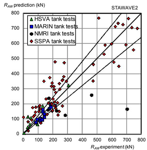
Figure 18 STAWave-1 and STAWave-2 correlated with model test results for various ship types, loading conditions and speeds in irregular head waves
