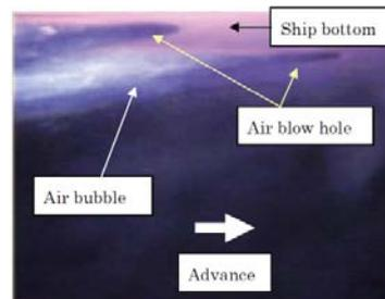
Figure 38 Air injection for full-scale ship
