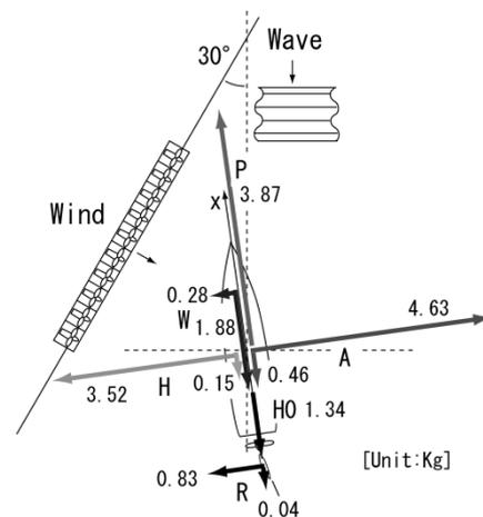
Figure 41 Force balances acting on the ship for external forces (wind speed: 4m/s and wave height: 0.12m, with wave length ship length ratio: 0.9).
