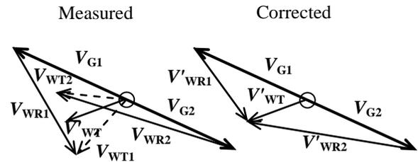
Figure 5 Averaging of measured wind vectors over two counter runs to derive the true wind vector
