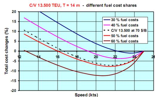
Figure 22 Total cost changes by speed reduction
