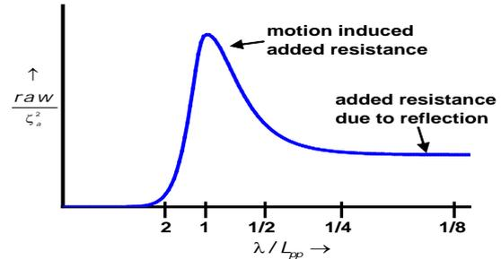
Figure 6 Added resistance in waves as function of wave length over ship length.
