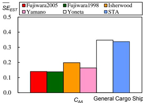
Figure 10 Averaged standard errors of longitudinal wind force coefficient for each ship type.
