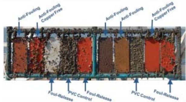
Figure 45 Fouling of several commercial formulations after 180 days static immersion (Swain, 2011).
