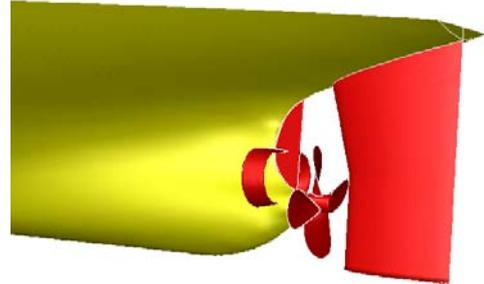
Figure 30 Configuration of Duct on VLCC
