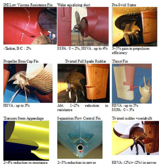
Figure 28 Different Energy-saving devices and gain rates
