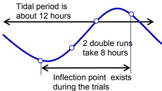
Figure 20 Relation on tidal velocity and trials for large low speed ship as VLCC.
