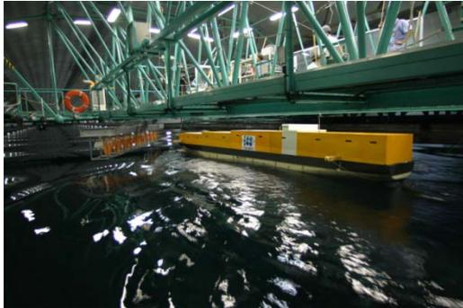
Figure 42 Photo of free-running model experiment of a container ship (from behind the ship).
