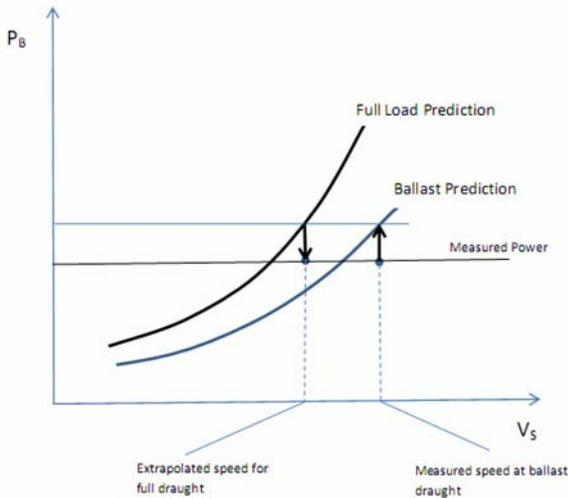
Figure 1 Extrapolation from measured values at sea trial condition to EEDI condition
