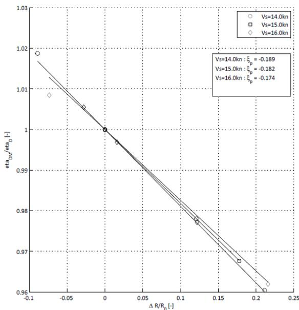
Figure 21 Example of load variation tests – relation between propulsion efficiency change and resistance increase.
