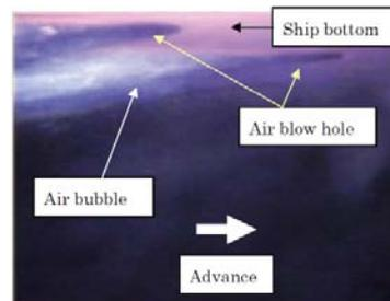
Figure 38 Air injection for full-scale ship
