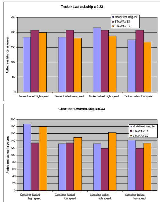
Figure 7 Added resistance in irregular head waves computed by STAwave 1 & 2 compared with results of large model tests for different speeds and loading conditions.
