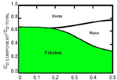
Figure 37 Resistance component –  $F_n$
