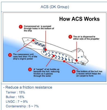
Figure 36 Resistance reduction by air
