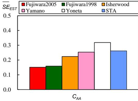
Figure 9 Averaged standard errors of longitudinal wind force coefficient (54 ships).
