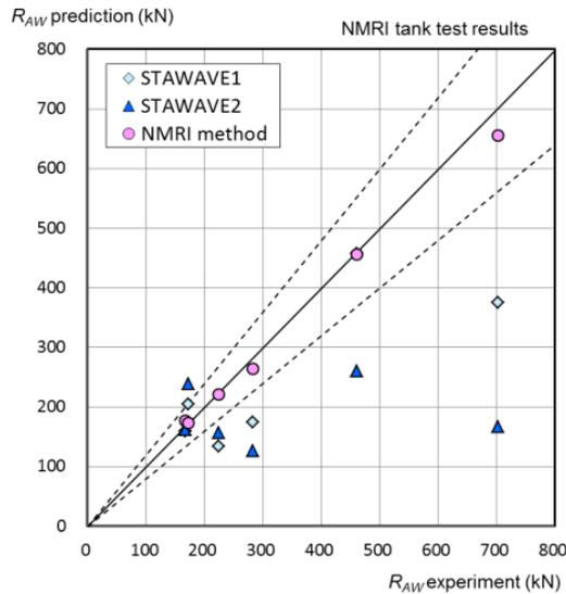
Figure 17 Wave correction methods compared with NMRI model test data; note NMRI model test results were used for the NMRI prediction method.
