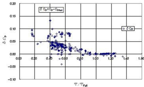
Figure 2 Variation of  $C_P - C_{P_{FULL}}$  as a function of the displacement ratio.
