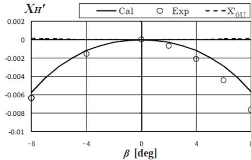
Figure 44 Longitudinal force due to ship drift (container ship,  $F_r=0.25$ )
