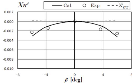
Figure 43 Longitudinal force due to ship drift (bulk carrier,  $F_r=0.15$ )
