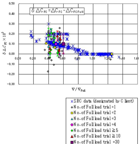
Figure 3 Variation of  $\Delta C_{FC}$  as a function of the displacement ratio.
