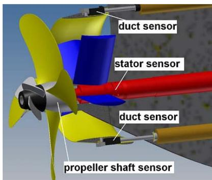
Figure 29 The sensors used to measure forces and moments.
