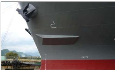
Figure 35 STEP installed in a RoRo vehicle carrier
