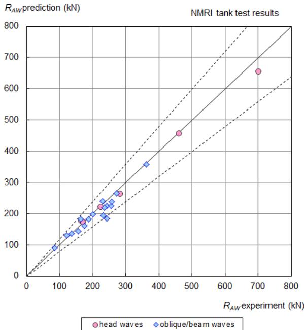
Figure 19 Comparison results for the NMRI method combined with empirical relation for the parameter estimation applied to oblique/beam waves.
