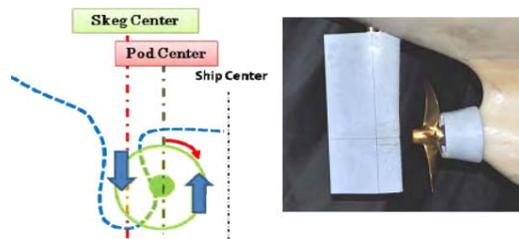
Figure 34 Concept of Reaction Pod (left) and Weather Adapted Duct (right)
