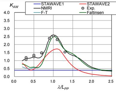
Figure 14 Bulk carrier ( $L=217\text{m}$ ,  $F_r=0.188$ ; Ballast)
