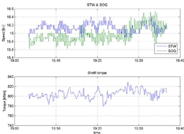
Figure 4 Speed through water and over ground and shaft torque measured on an 1800 TEU container vessel in 4 m significant wave height (Courtesy; Vroon)
