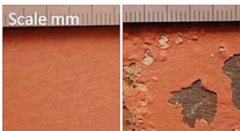
Figure 46 Ship hull coating condition. Left: 3 year self-polishing copper  $70\mu\text{m}$  AHR. Right: 11 year hybrid copper  $264\mu\text{m}$  AHR plus damage (Swain, 2011).
