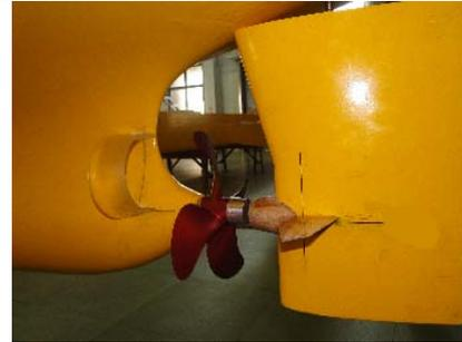
Figure 33 Combined energy-saving devices
