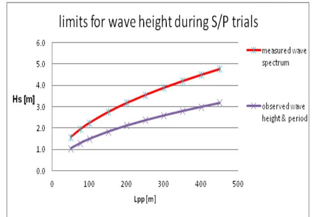
Figure 8 New limits for significant wave height
