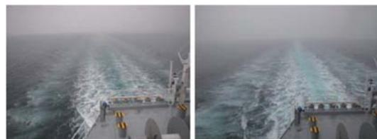
Figure 39 Wake flow without air injection (left) and with air injection (right)
