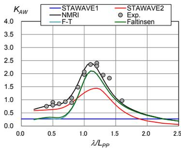
Figure 12 Car carrier ( $L=190\text{m}$ ,  $F_r=0.249$ ; Full)
