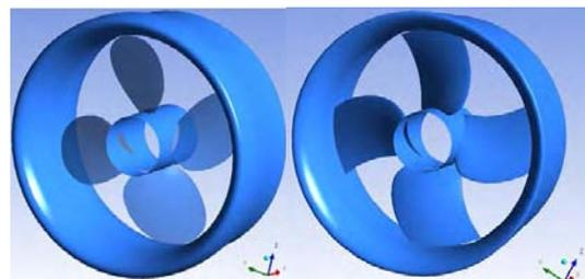
Figure 23 ducted propeller (left: original, right, optimized )
