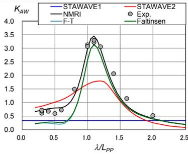
Figure 11 Container ship ( $L=300\text{m}$ ,  $F_r=0.247$ ; Full)
