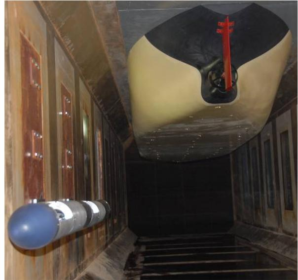
Figure 5. SPIV measurement setup in the LCC at CSSRC.
