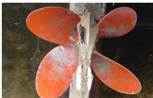
Figure 1.2- The propeller of “Bernicia” after 12 months in service after coating. 95% of the coating is intact, except some detachment of the blade edges. Light slime fouling is present on the inner half of the blades (grey material on the red coating is the dried biofilm). This could be easily removed by hand or with a damp cloth (Mutton et al., 2005).
