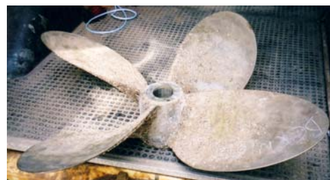
Figure 1.1- The propeller of “Bernicia” after 14 months in service before coating. Hard shell fouling is present to half the blade radius (Mutton et al., 2005).
