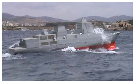
Figure 1.5- Testing at high model sea states.
