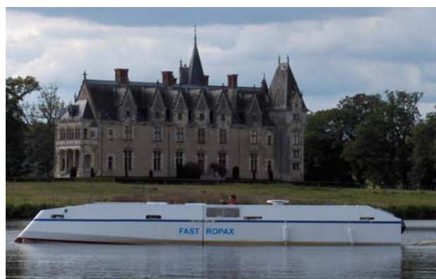
Figure 1.7- VRSHIPS/ROPAX testing platform.
