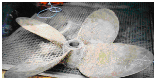
Figure 1.2- The propeller of “Bernicia” after 14 months in service before coating. Hard shell fouling is present to half the blade radius (Mutton et al., 2005).
