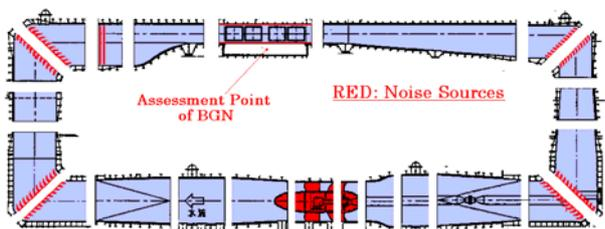
Figure 1.20- Divided elements of FNS for Acoustic Power Balance Method.
