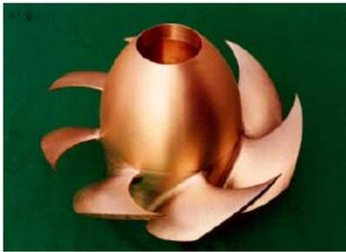
Figure 1.18- Impeller geometry (model).
