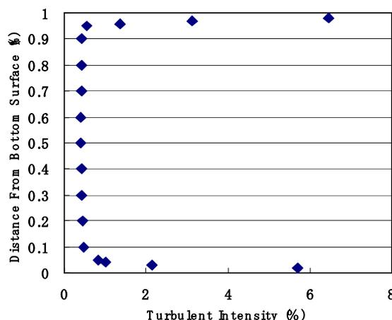
Figure 1.17- Turbulence intensity at the test section.
