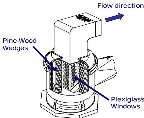
Figure 1.19- Noise Absorbing Tank.
