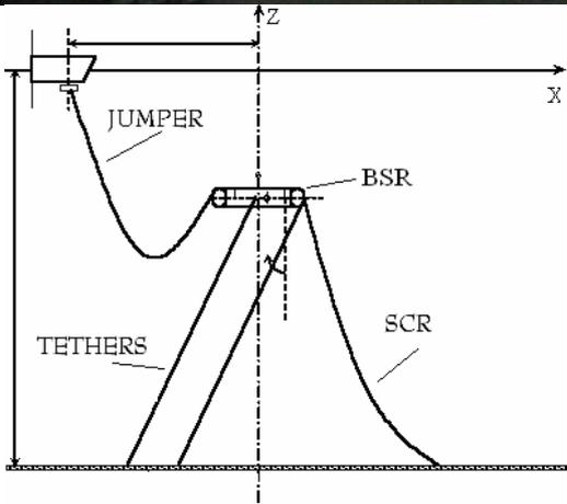
Figure 1.8- BSR, Bóia de Suporte de Riser (Riser Support Buoy).
