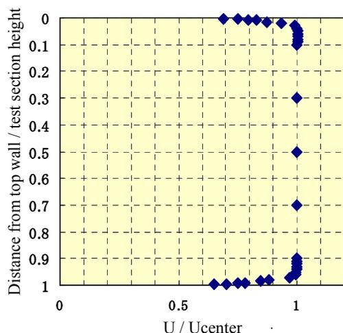
Figure 1.16- Velocity profile at the test section.
