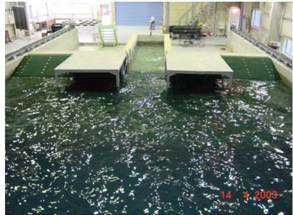
Figure 1.2: Front wave absorber.
