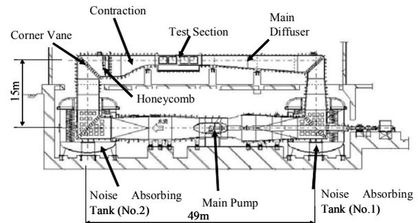
Figure 1.15- FNS overall geometry.
