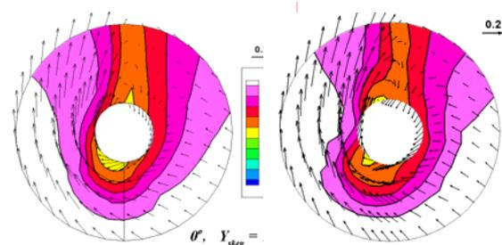
Figure 9.9- Comparison of wake distribution between computation and measurement.
