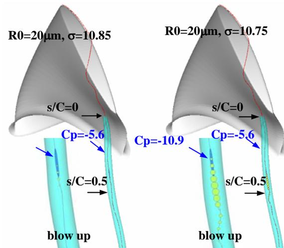
Figure 8.7- Bubble trajectories and size variations during bubble capture by the two-vortex system (Hsiao and Chahine, 2004b).
