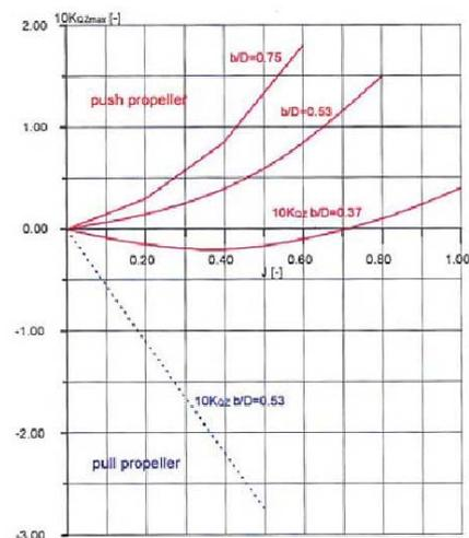
Figure 6.10- Maximum moment coefficient \$K\_{Qz}\$ of an azimuthing thruster with ducted propeller (Voytkunskiy, 1985).
