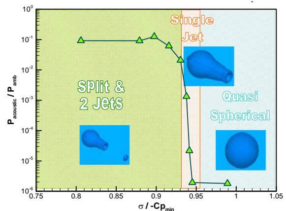
Figure 8.3- Acoustic pressure emitted by a bubble in a vortex (Choi and Chahine, 2003).
