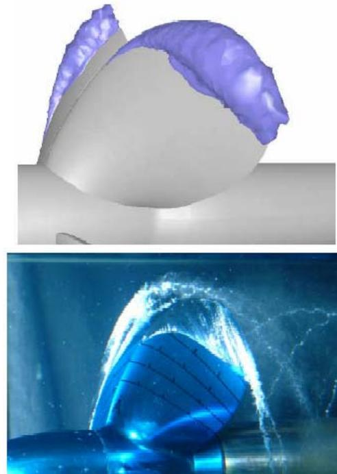
Figure 8.9- Cavity on blades at  $J=0.2$  and  $\sigma=2.0$  numerical simulation (top), experiment (bottom) (Rhee et al., 2003).
