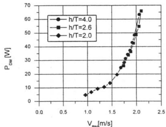
Figure 7.4- Delivered power versus blockage speed (Jiang, 2001).
