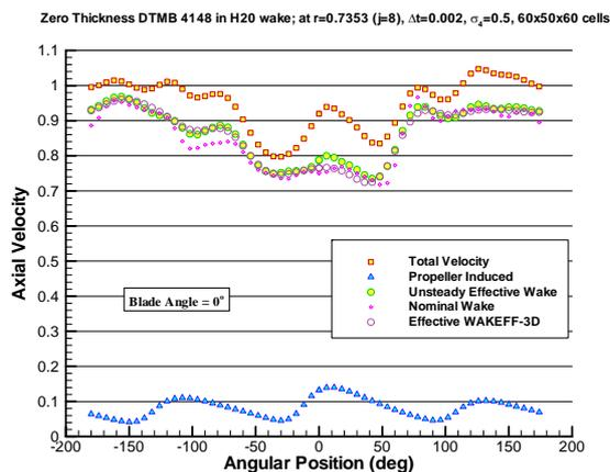
Figure 8.2- The axial velocity distributions when the key blade is at 0 deg. DTMB4118 propeller in non-axisymmetric inflow (Choi and Kinnas, 2003).
