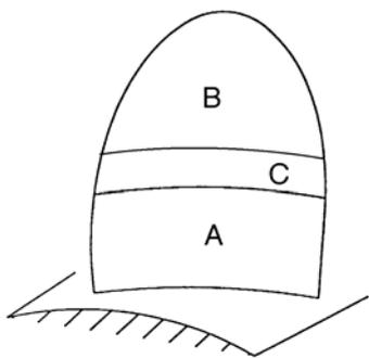
Figure 2.5- Concept of the Trans-Cavitating Propeller.
