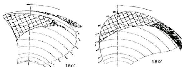
Figure 6.3- Comparison of observed cavitation extent between two impeller models (Yamasaki et al., 2000).
