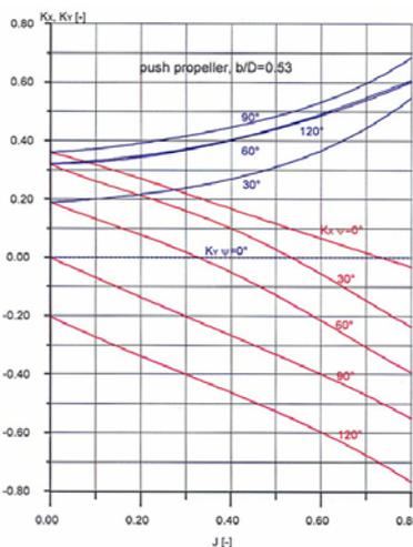
Figure 6.8- Thrust coefficient of an azimuthing thruster with a ducted push-propeller (Voytkunskiy, 1985).
