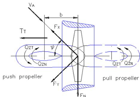
Figure 6.7- Forces and moments at an azimuthing thrusters with a ducted pull or push propeller (Voytkunskiy, 1985).
