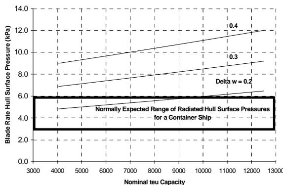
Figure 9.2- Estimation chart of blade-rate hull pressure fluctuations (Carlton, 2001).
