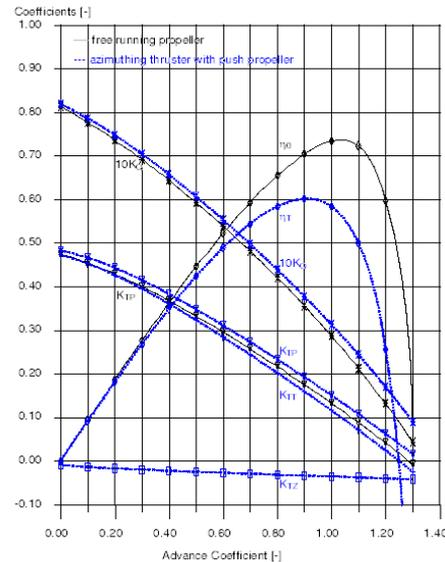
Figure 6.6- Open water characteristics of Wageningen B4.50 without and with z-drive housing (Heinke H.-J., 1998).
