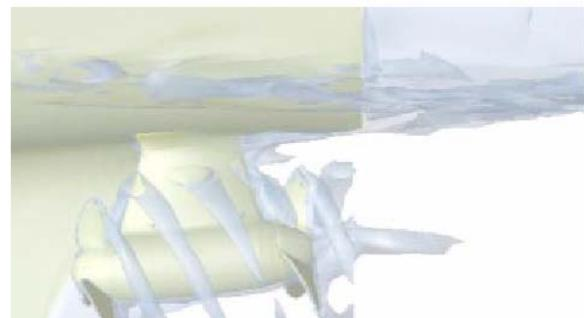
Figure 5.3- Predicted vorticity field around a podded propulsor by RANS (Streckwall and Tigges, 2003).
