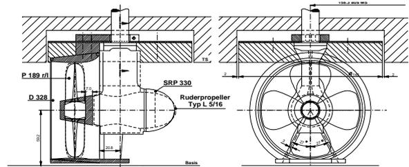
Figure 7.6- Rudder in an integrated nozzle.
