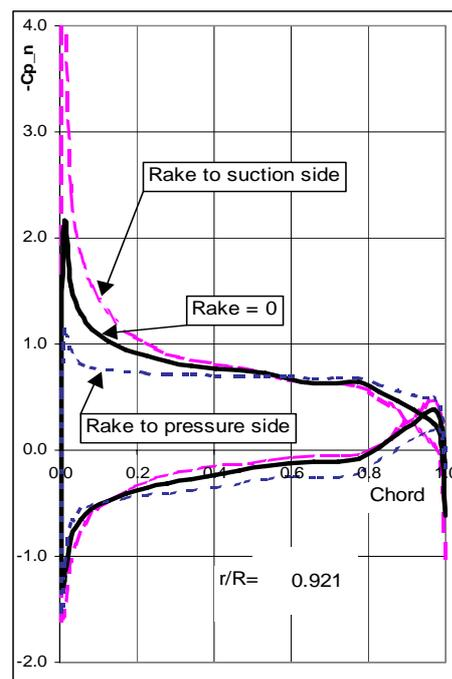
Figure 2.3- Comparison of the pressure distribution on a propeller with three different tip rakes (Dang, 2004).
