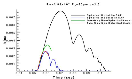
Figure 8.5- Comparison of the bubble radius versus time for the spherical models (the conventional and the SAP model) and the 3-D 1-way and 2-way UnRANS computations (Hsiao and Chahine, 2004a).
