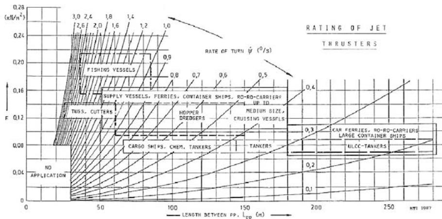
Figure 6.1- Lateral thruster design figure (Brix, 1993).
