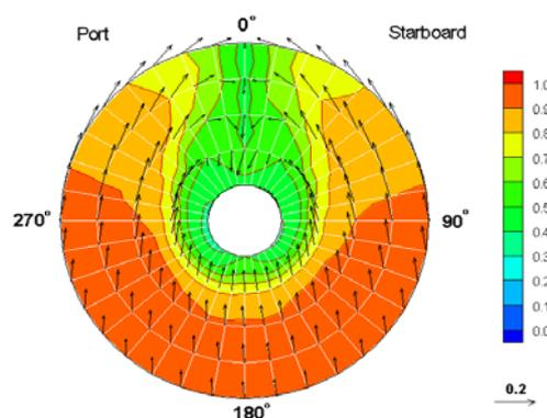
Figure 9.1- Estimated full-scale wake of a typical mega-containership (Kume et al., 2004).
