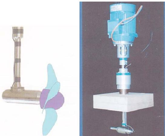
Figure 6.5- MARIN (left) and FORCE Technology (right) model thruster measuring system (Cornel, 2000 and FORCE Technology, 2001).
