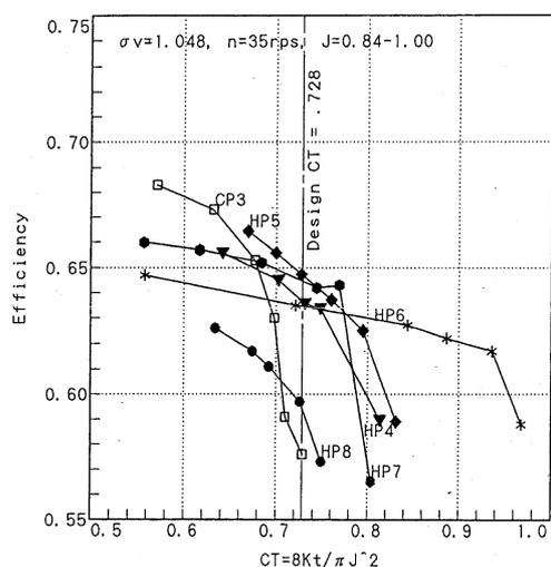
Figure 2.6- Propeller open water performance for the 35 knots case.
