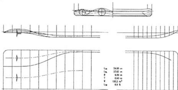
Figure 7.5- Four-propeller pusher with an inner tunnel height of 0.90m and an outer tunnel height of 0.75m.
