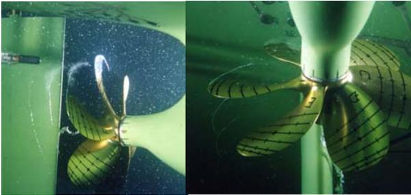
Figure 9.5- Typical cavitation pattern on large propeller of a mega-containership.
