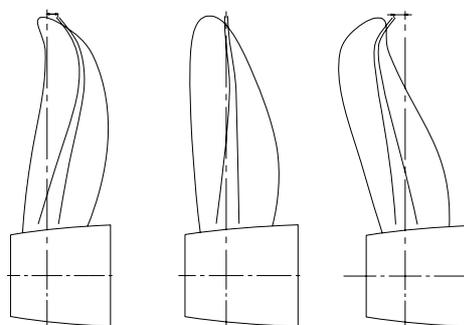
Figure 2.2- Three different tip rakes (from left: rake to pressure side, no rake, rake to suction side) (Dang, 2004).
