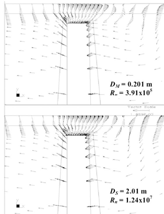
Figure 5.2- RANS predictions of the velocity distribution in the gap region of a ducted propeller (Abdel-Maksoud and Heinke, 2002).
