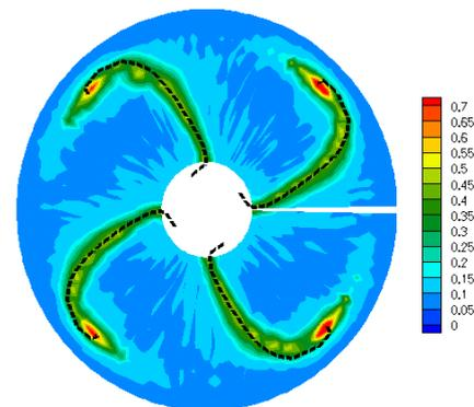
Figure 5.1- Propeller trailing wake predictions by BEM (dashed black lines) compared to vorticity field derived from LDV measurements (Greco et al., 2004).
