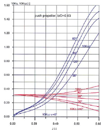
Figure 6.9- Torque coefficient of an azimuthing thruster with a ducted push-propeller (Voytkunskiy, 1985).
