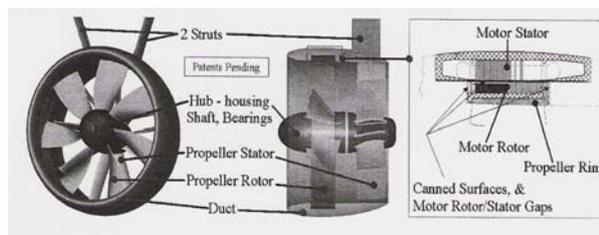
Figure 2.4- Rim-driven propulsor (Van Blarcom et al., 2004).
