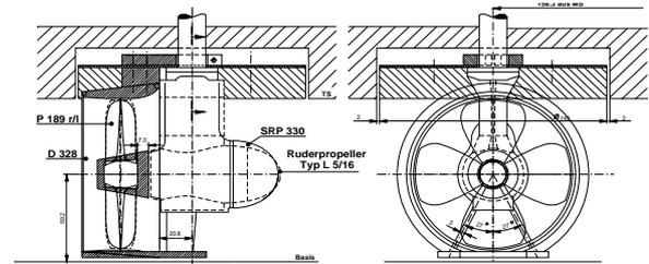
Figure 7.6- Rudder in an integrated nozzle.
