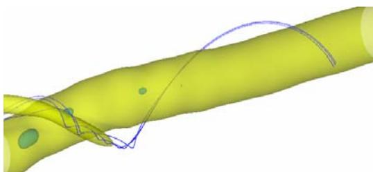
Figure 8.6- Interaction between two vortices resulting in ejection of initially trapped nuclei out of the main vortex (Hsiao and Chahine, 2003).
