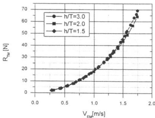
Figure 7.3- Total model resistance versus effective speed (Jiang, 2001).
