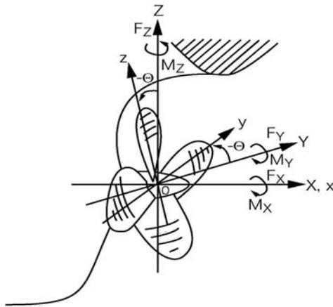
Figure 9.6- Definition of coordinate system on bearing force.
