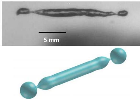
Figure 8.4- Bubble behaviour in a vortex flow field. 3-D view of the bubble just before splitting observed at University of Michigan (upper) and predicted by 2DYNAPS<sup>®</sup> (lower) (Rebow et al., 2004).
