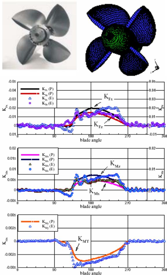
Figure 8.8- Comparison of predicted (P) and measured (E) blade forces for SPP model 841-B.  $J_A=1.2$ ,  $h/D=0.33$  (Young and Kinnas, 2002).
