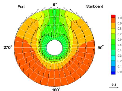
Figure 9.1- Estimated full-scale wake of a typical mega-containership (Kume et al., 2004).
