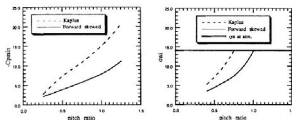
Figure 6.4- Comparison of minimum pressure (left) and cavitation inception speed (right) between two impeller models (Ohshima, 2001).
