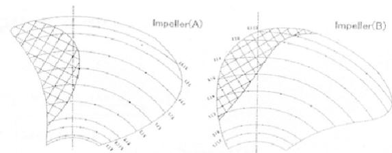
Figure 6.2- Comparison of calculated cavitation extent between forward skew (A) and backward skew (Yamasaki et al., 2000).
