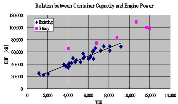
Figure 9.3- Trend on main engine power for current and future containerships.
