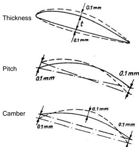
Figure 4.1- Description of the variations in propeller geometry.
