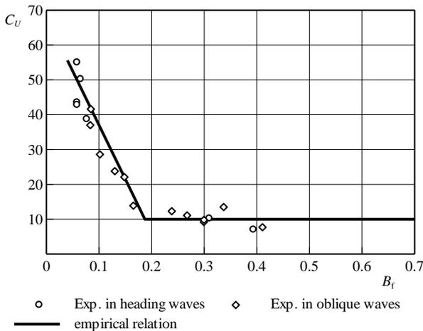
Fig.D-4 Relation between the coefficient of advance speed on added resistance due to wave reflection and the bluntness coefficient for conventional hull form above water.
