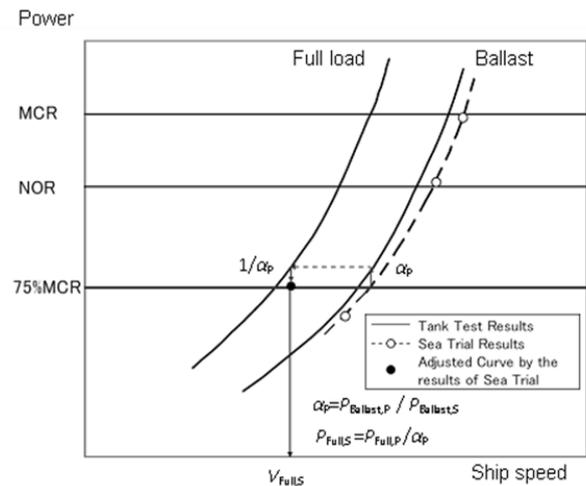
Fig.E-1 An example of ship speed adjustment using power ratio.
