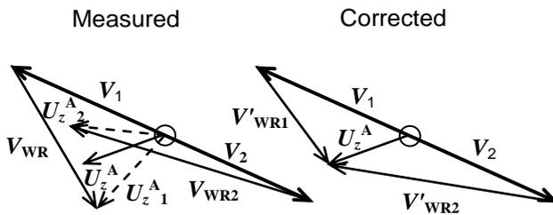
Figure B-1 True wind vectors and relative wind vectors.
