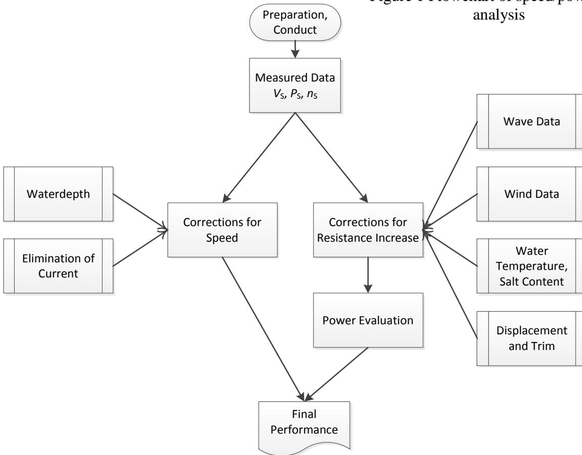
In the following chapters details of the methods are given. For wave and wind corrections the methods depend on the level of information which is available to the conducting party of the speed/power sea trials. The analysis and correction method to be followed is prescribed below and summarized in Table 1.
