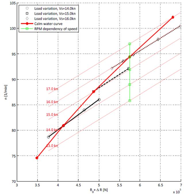
Figure A.3 Relation between propeller rate and speed change
