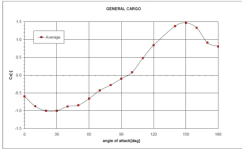
Fig.C-1 Wind resistance coefficients for various ship types<sup>(19)</sup>.
