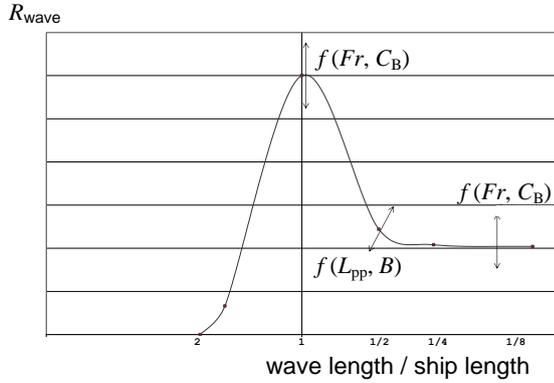
Fig.D-2 Parametric transfer function of meanresistance increase in regular waves.
