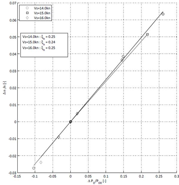
Figure A.2 Relation between propeller rate and power increase
