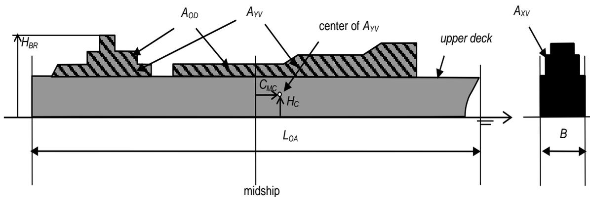
Figure C.2 Input parameters for regression formula by Fujiwara
