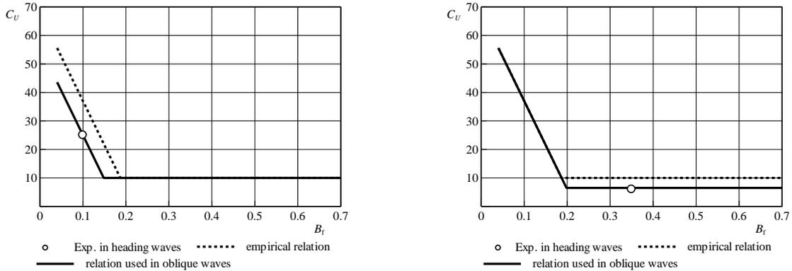
Fig.D-5 Shift of the empirical relation in oblique waves (upper; for fine ship  $B_f < 58/310$ , lower; for blunt ship  $B_f \geq 58/310$ ).
