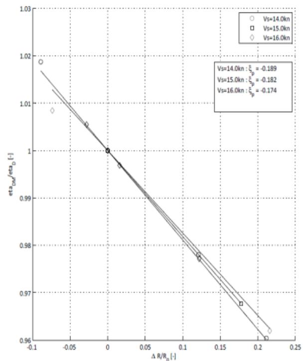
Figure A.1 Relation between propeller efficiency and resistance increase
