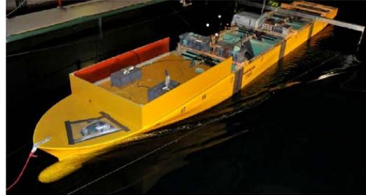
Figure 2. Segmented Elastic Model with Transducers at Segments (Wu, 2010).
