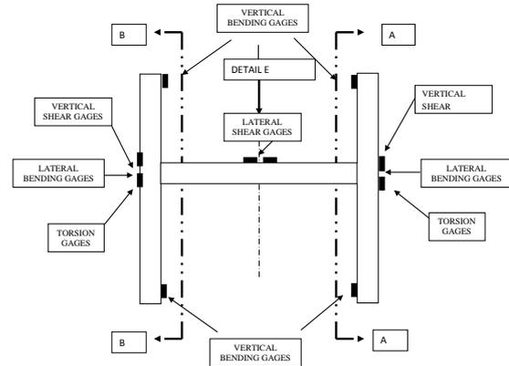
Figure 3. Possible Strain Gage Measurement for Internal Elastic Strength Bar (Dinsbacher, 2010).
