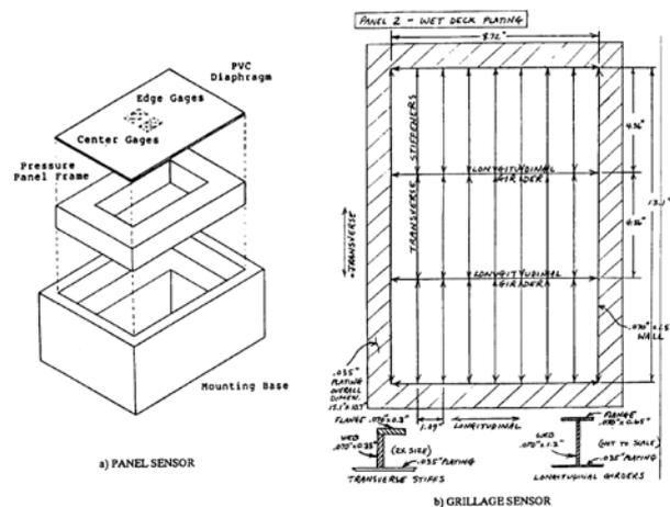
Figure 8. Example of Panel and Grillage Sensors (Dinsenbacher, 2010).
