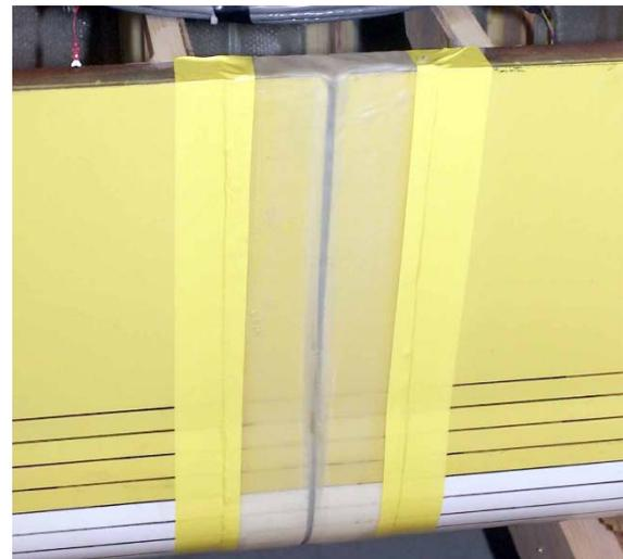
Figure 6. Example of Segment Sealant (Hayden, 2009).
