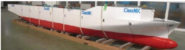
Figure 1. Elastic Segmented Model with Internal Back-spline Beam (Miyake, 2009).
