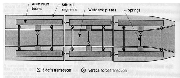
Fig. 2 – Set-up of a hydroelastic catamaran model.
