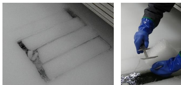
Figure 14: Ice thickness measurements with calliper
