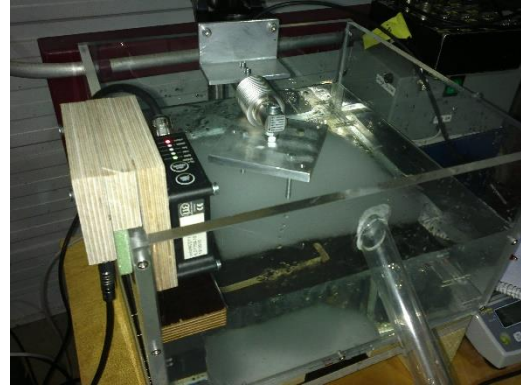
Figure 7: Ex-situ density measurement setup (Option B)
