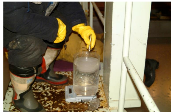
Figure 8: Force balance measurement without displacement recording (Option C)
