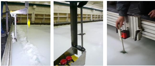
Figure 15 Ridge-profiling device to determine keel depth and sail height
