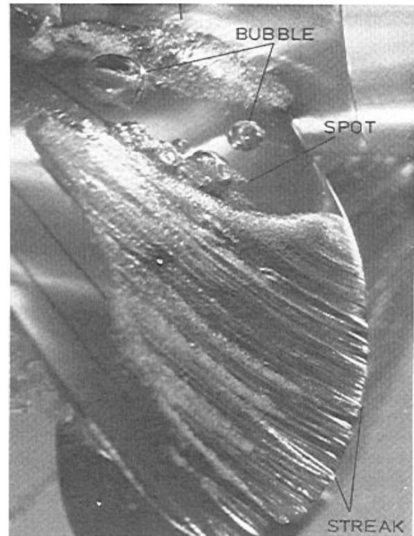
Figure 2 Leading edge, large bubble and root cavitation
