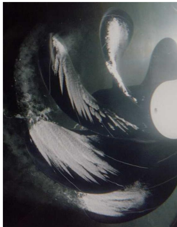
Figure 4 Small bubble and streak cavitation
