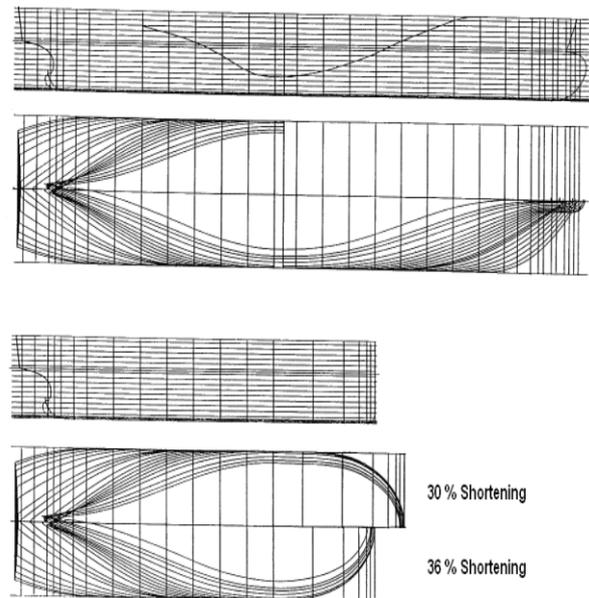
Fig. 2: Shortening of a Container Vessel Model
