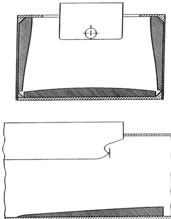
Fig. 1: Flow Liners in a Cavitation Tunnel
