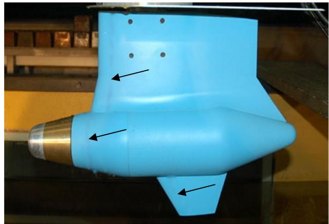
Figure 11 Typical turbulence stimulator arrangement applied to pod housing
