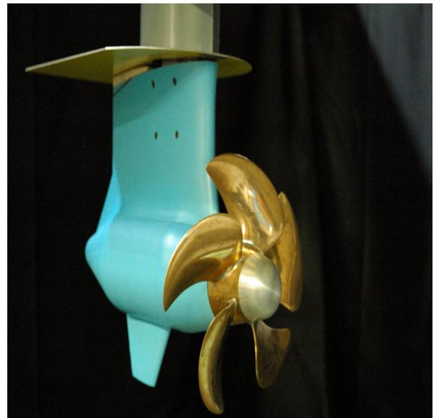
Figure 5 Typical pod unit open water test set-up
