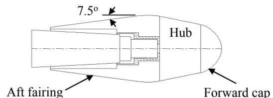
Figure 2 Example of hub geometry for an open water test with a pulling type
