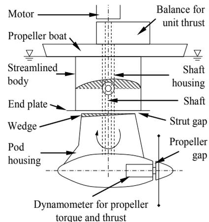
Figure 4 Typical pod unit open water test set-up
