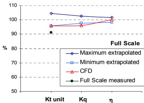
Figure 17 Range of performance coefficients extrapolated to full scale by different model basins
