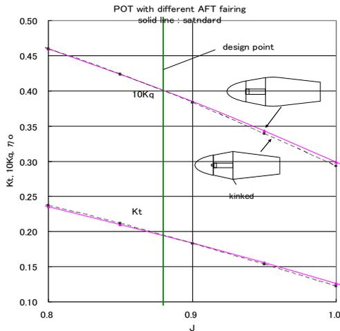
Figure 3 Effect of aft fairing on propeller open water characteristics
