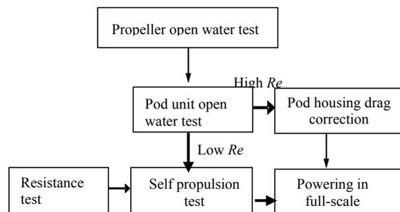
Figure 1 Flow diagram of power prediction of a vessel with podded propulsion
