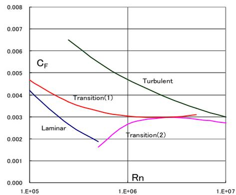
Figure 13 Frictional coefficients of laminar, transition and turbulent
