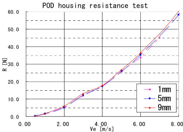
Figure.8 Pod resistance of table 4 with different strut gaps
