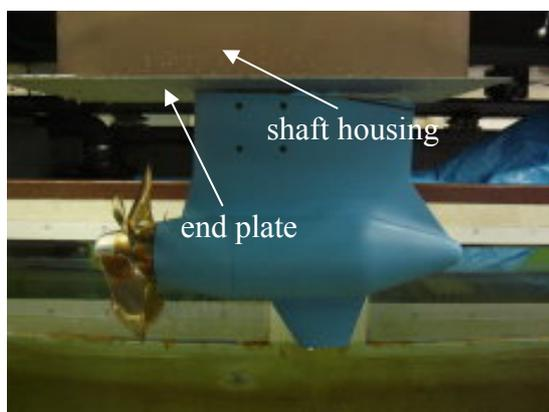
Figure 6 Shaft housing and end plate
