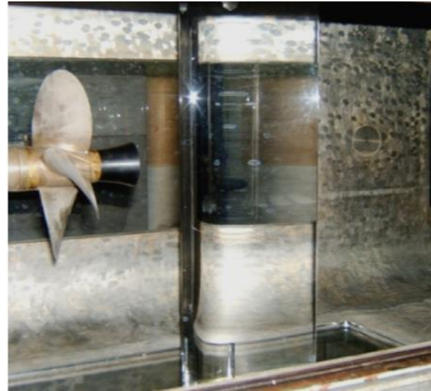
Figure 6. Use of Perspex in order to avoid light reflection (Felli et al., 2011)
