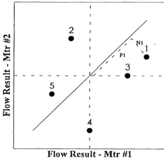
Figure 4: Youden plot for flow meter test
