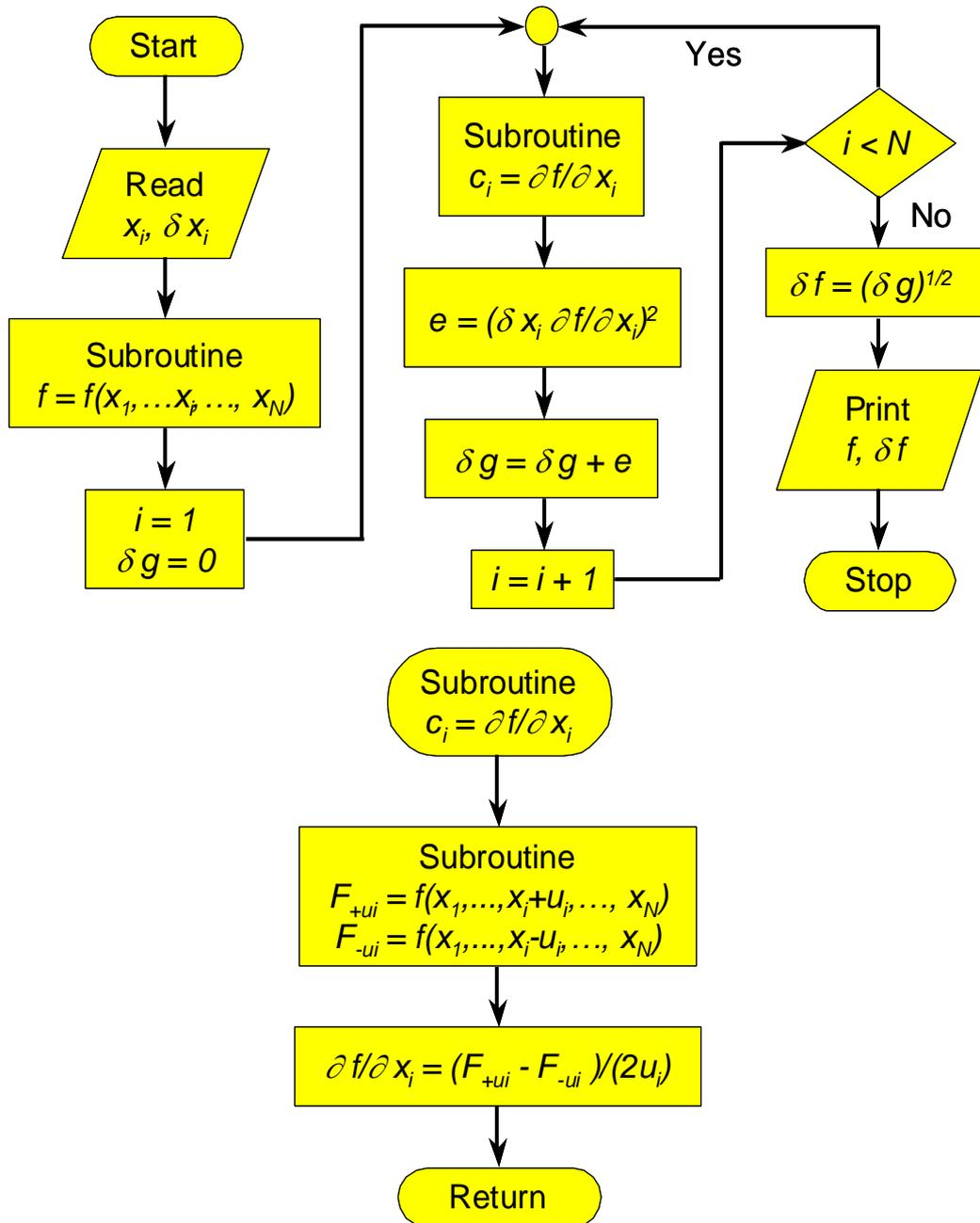
Figure 2: Flow chart for numerical determination of sensitivity coefficients (Moffat, 1982)
