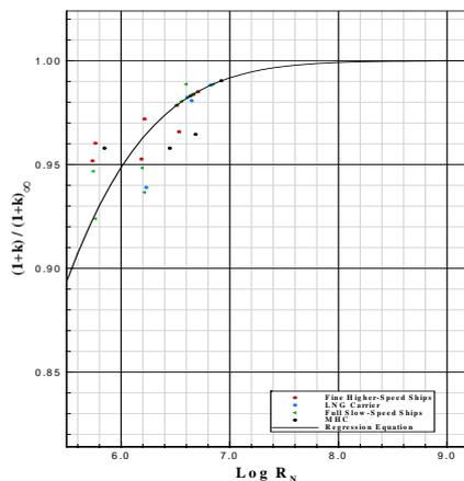
Figure. 6 Form factor correction factor curve
