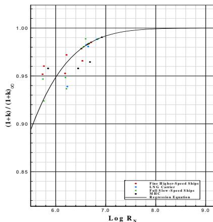
Figure. 6 Form factor correction factor curve
