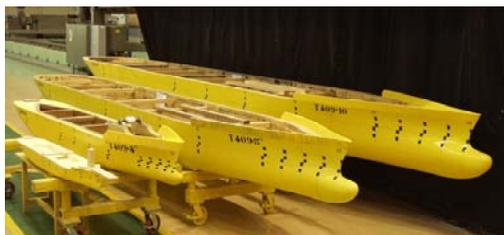
Figure.3 Models of 155,000 m<sup>3</sup> LNG carrier.
