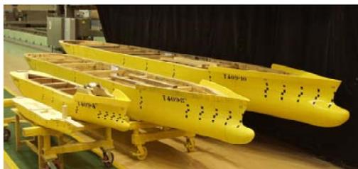
Figure.3 Models of 155,000 m<sup>3</sup> LNG carrier.
