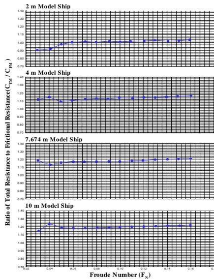
Figure. 4 Low-speed resistance test result of 155,000 m<sup>3</sup> LNG carrier
