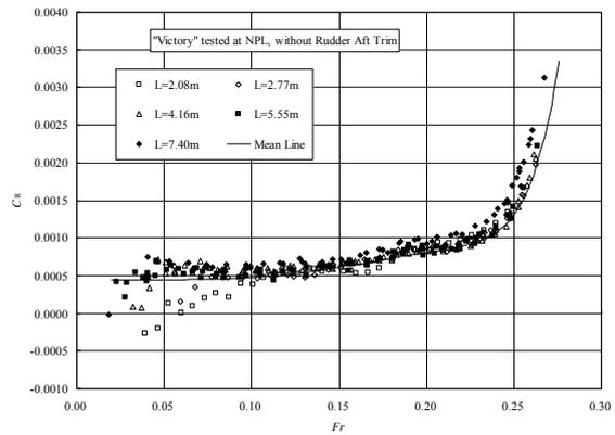
Figure.8 Simply analysed results of “Victory” Geosim test results presented by Hughes
