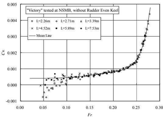
Figure.7 Analysed results of “Victory” Geosim test results presented by van Lammeren et.al.
