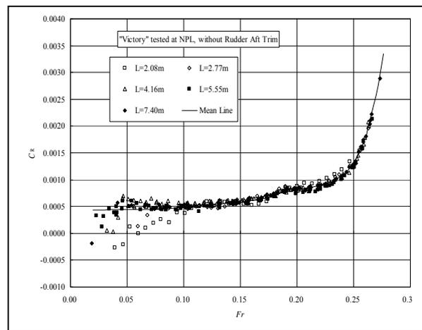
Figure.9 Analysed results of “Victory” Geosim test results presented by Hughes (after blockage correction)
