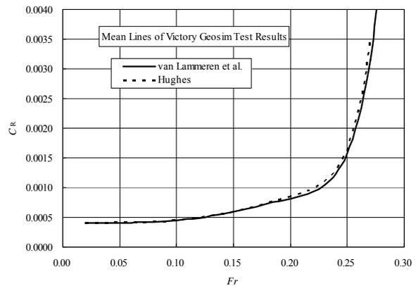
Figure.10 Comparison of mean lines derived from the two “Victory” Geosim test results
