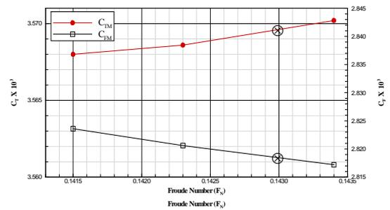
Figure. 5 Resistance test result in the vicinity of the design speed for 317,000 TDW VLCC
