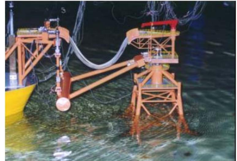
Fig. 6 Model test of a tower yoke mooring system
