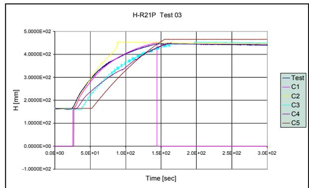
Figure 3.11 Water Level for Compartment R21P
