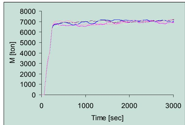
Figure 3.22 Flood Water Mass Versus Time,  $H_s = 4$  m, Damage Case D2
