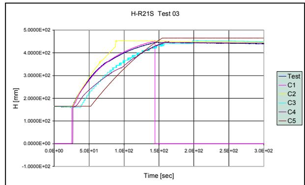
Figure 3.10 Water Level for Compartment R21S
