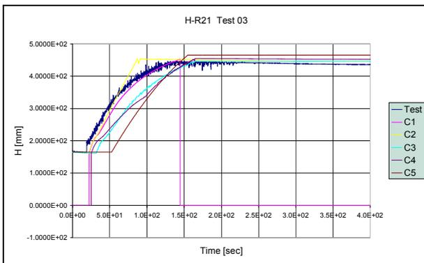
Figure 3.9 Water Level for Compartment R21
