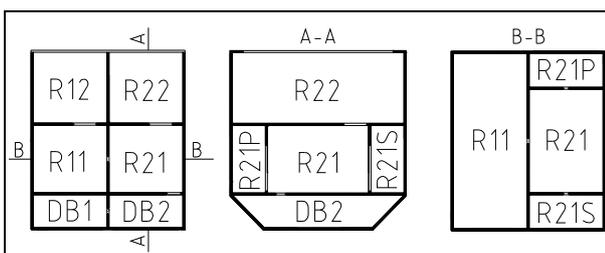
Figure 3.5 Internal Compartments
