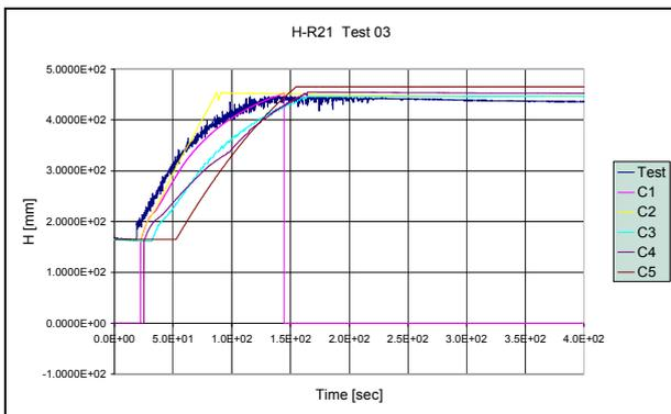
Figure 3.9 Water Level for Compartment R21
