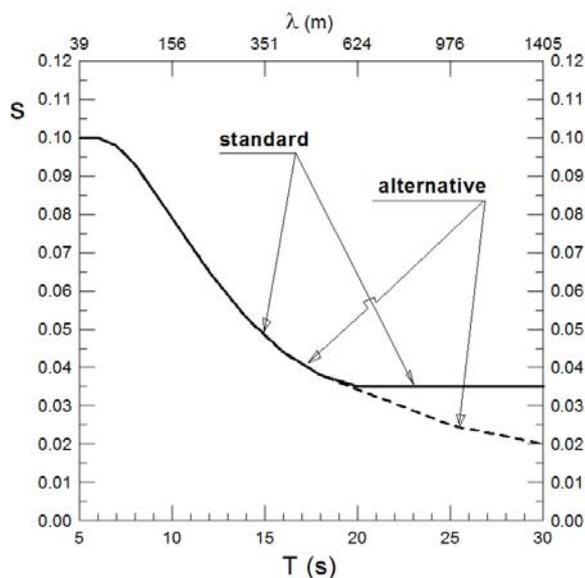
Figure 4.1 Wave steepness as a Function of Roll Natural Period as in Standard Weather Criterion and as Adopted in the Alternative Assessment with an Experimental Basis
