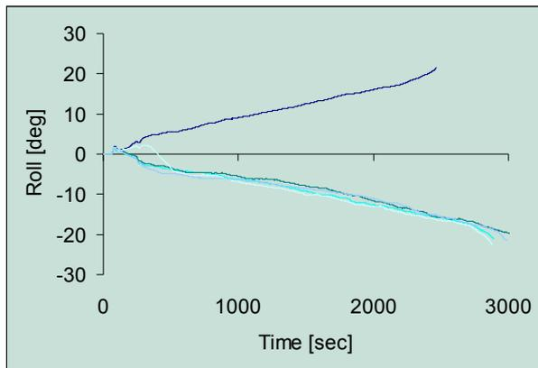
Figure 3.19 Roll Versus Time,  $H_s = 4$  m, Damage Case D1
