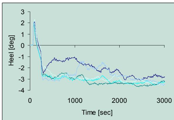
Figure 3.20 Roll Versus Time,  $H_s = 4$  m, Damage Case D2
