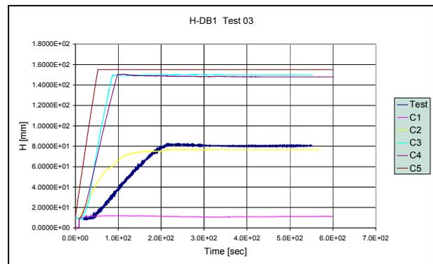
Figure 3.6 Water Level for Compartment DB1
