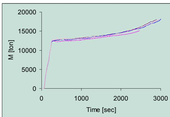
Figure 3.21 Flood Water Mass Versus Time,  $H_s = 4$  m, Damage Case D1
