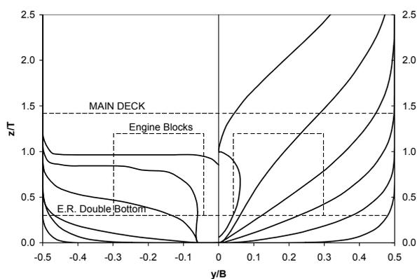
Figure 3.1 The Body Plan of the Study Ship
