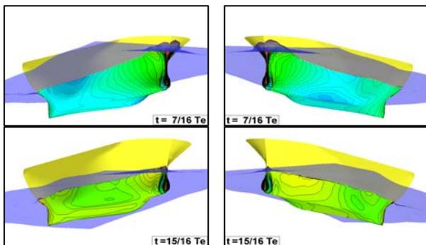
Figure 9: Computed pressure distributions on a container ship,  $Fr=0.25$ ,  $\chi=120deg$ ,  $\lambda/L=1.0$
