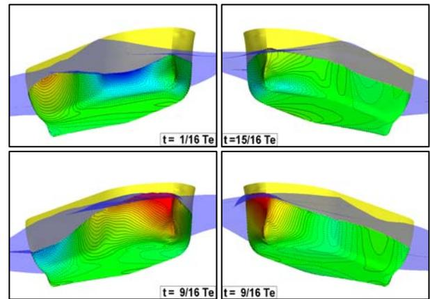
Figure 10: Computed pressure distributions on a VLCC (Full load condition),  $Fr=0.15$ ,  $\chi=120deg$ ,  $\lambda/L=0.5$
