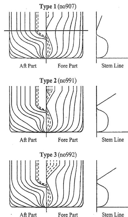
Figure 7: Body plan of VLCC variants
