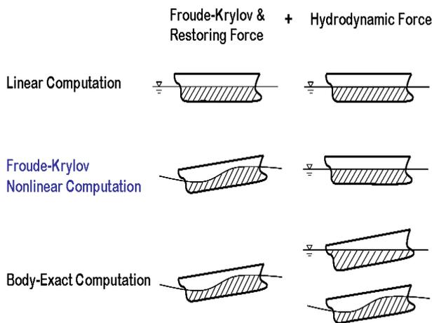
Figure 1: Summary of linear and nonlinear computational methods for ship motion (Singh and Sen, 2007)
