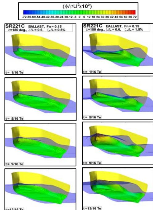
Figure 11: Computed pressure distributions on a VLCC (Ballast cond.),  $Fr=0.15$ ,  $\chi=180deg$ ,  $\lambda/L=0.6$
