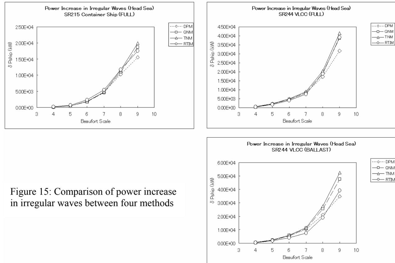
Figure 15: Comparison of power increase in irregular waves between four methods
