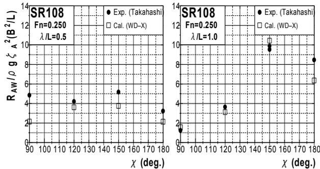
Figure 12: Added-resistance coefficients for a container ship,  $\lambda/L=0.5$  and  $1.0$
