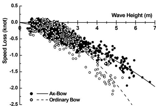
Figure 5: Comparison of speed loss at sea
