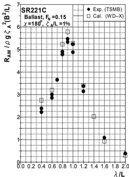
Figure 14: Added-resistance coefficients for a VLCC (Ballast cond.),  $Fr=0.15$ ,  $\chi=180\text{deg}$
