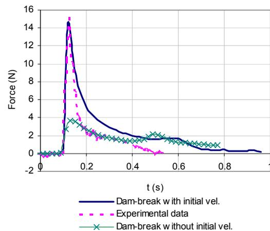
Figure 4: Comparison of horizontal load for an S-175 container ship at  $Fr = 0.3$ ,  $H = 8.0\text{m}$  and  $T = 12\text{s}$ . Varyani et al. (2004).
