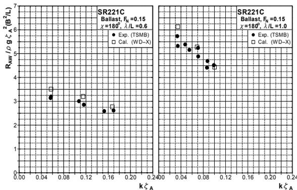
Figure 13: Added-resistance coefficients for a VLCC (Ballast cond.),  $Fr=0.15$ ,  $\chi=180\text{deg}$ ,  $\lambda/L=0.5$  and  $1.0$  vs. wave slope
