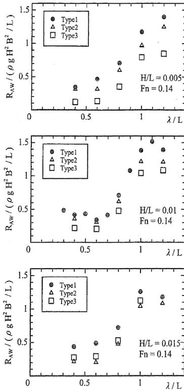
Figure 8: Influence of above-water bow forms on computed added resistance.
