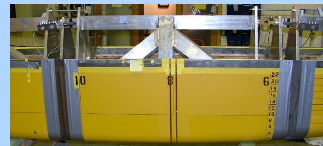
Flexible Connections for Non-Backspline Elastic Segmented Model (Drummen, 2007).
