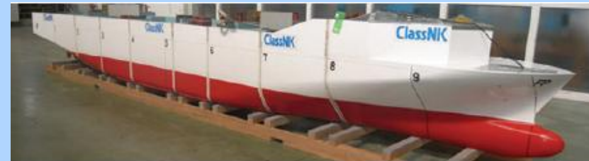
Elastic Segmented Model with Internal Backspline Beam (Miyake, 2009).
