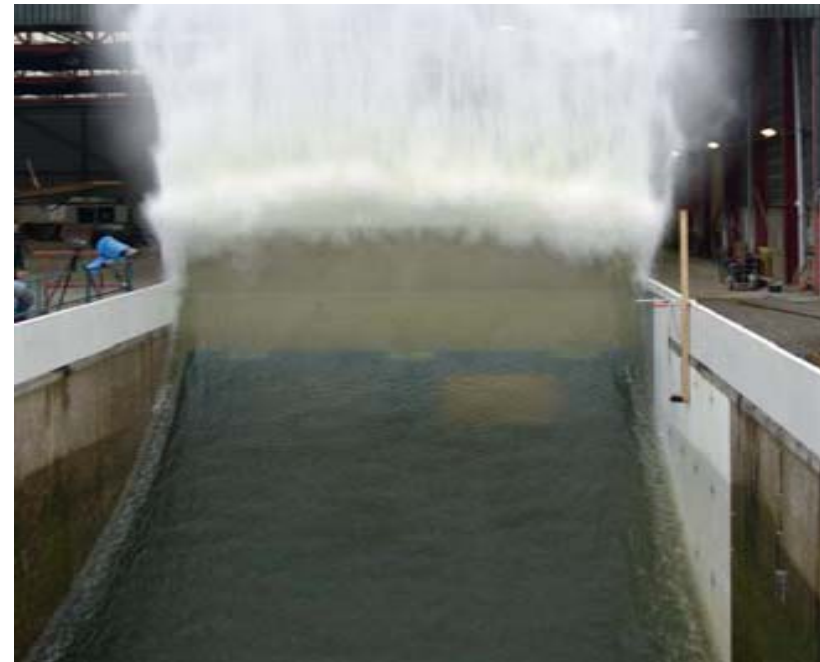
Figure 2.5.3: Full Scale Impact Tests on NO96 Elements in the Delta Flume, SLOSHEL JIP (Kaminski & Bogaert, 2009)
