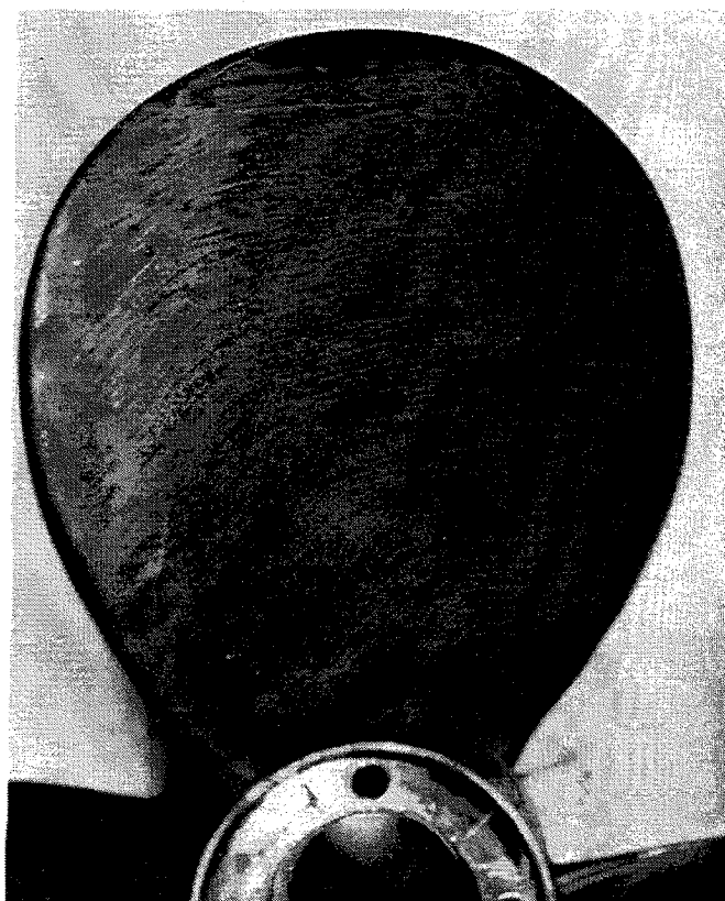
Figure 2.5 Flow Visualization Test: Paint Test Suction Side
