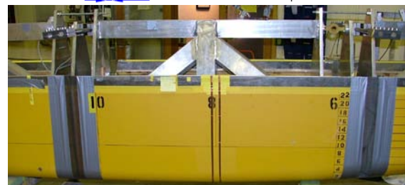
Figure 4. Instrumented Flexible Connections for Non-Backspline Elastic Segmented Model (Drummen, 2007).
