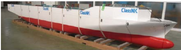
Figure 1. Elastic Segmented Model with Internal Backspine Beam (Miyake, 2009).
