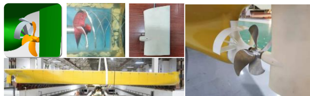
Figure 80 Energy saving model test of 230K DWT Ore Carrier
