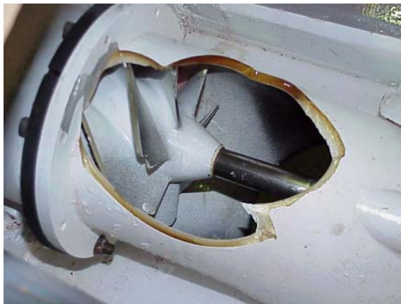
An unintended close look into the damaged waterjet for self propulsion tests.
