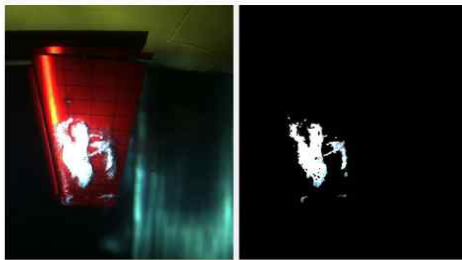
Quantification of cavitation amount using image processing
