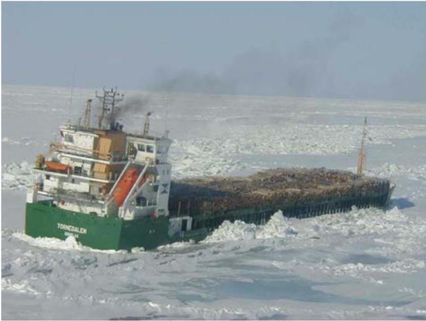
Figure 6: A ship stuck in compressive ice
