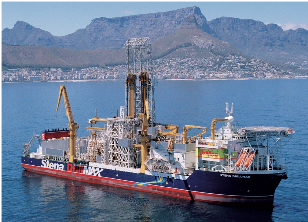
Figure 9-1: A typical modern Drill Ship with dual heads
