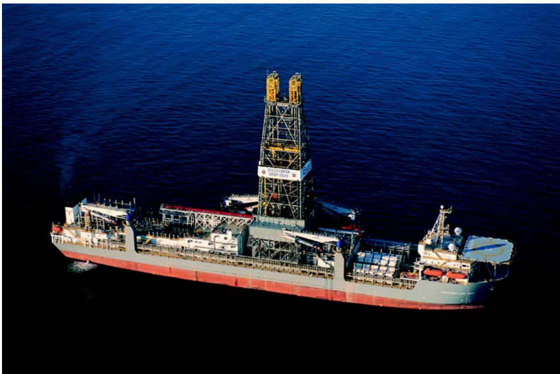
Figure 9-4: Ultradeepwater drill ship Transocean Discover class Discover Deep Seas. There are three of these type of units, which are 254.5 m long with a power rating of 52,000 hp and displacement of 92,800 t. Note the dual crown block for dual activity. Courtesy Transocean.
