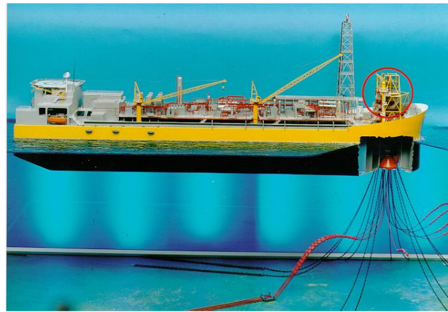
Single Point Mooring
