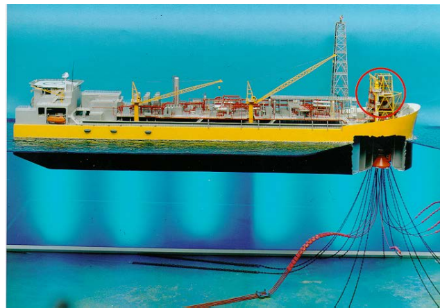
Single Point Mooring
