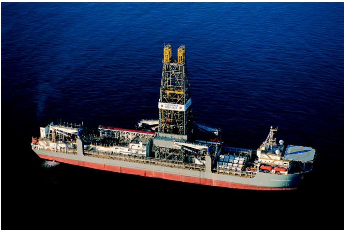
Figure 9-4: Ultradeepwater drill ship Transocean Discover class Discover Deep Seas. There are three of these types of units, which are 254.5 m long with a power rating of 52,000 hp and displacement of 92,800 t. Note the dual crown block for dual activity. Courtesy Transocean.
