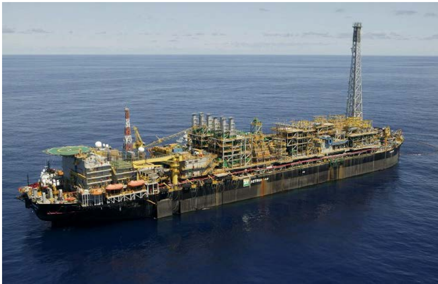
Figure 9-5: FPSO (Turret at the left end of picture)
