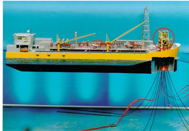
Single Point Mooring
