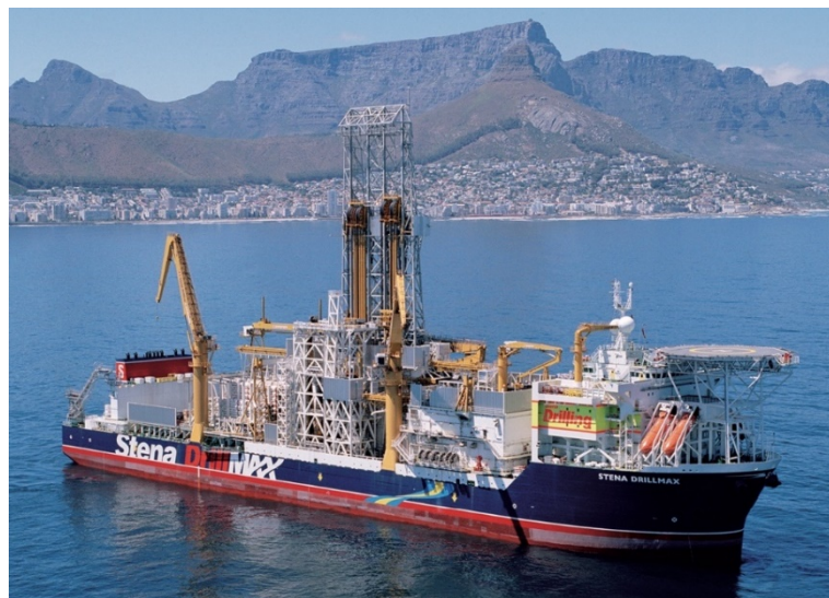
Figure 26: A typical modern Drill Ship with dual heads
