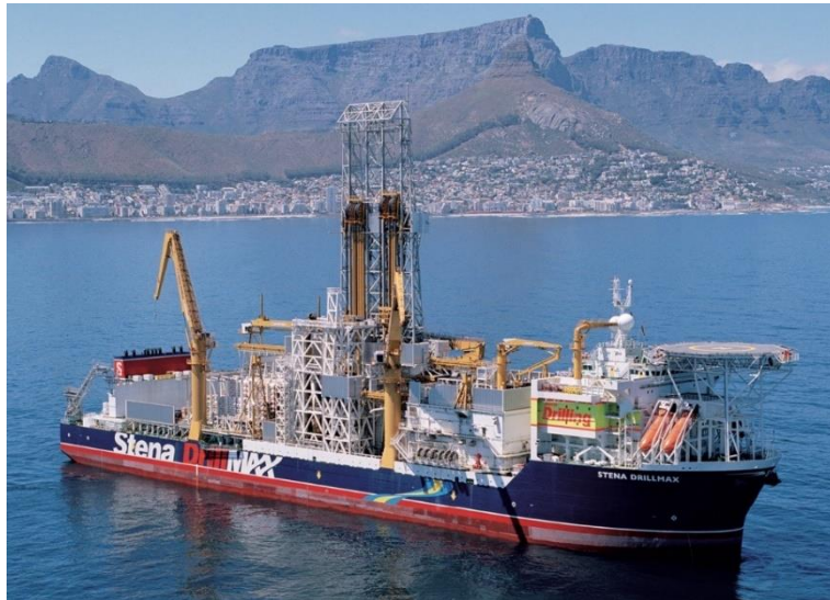
Figure 26: A typical modern Drill Ship with dual heads.
