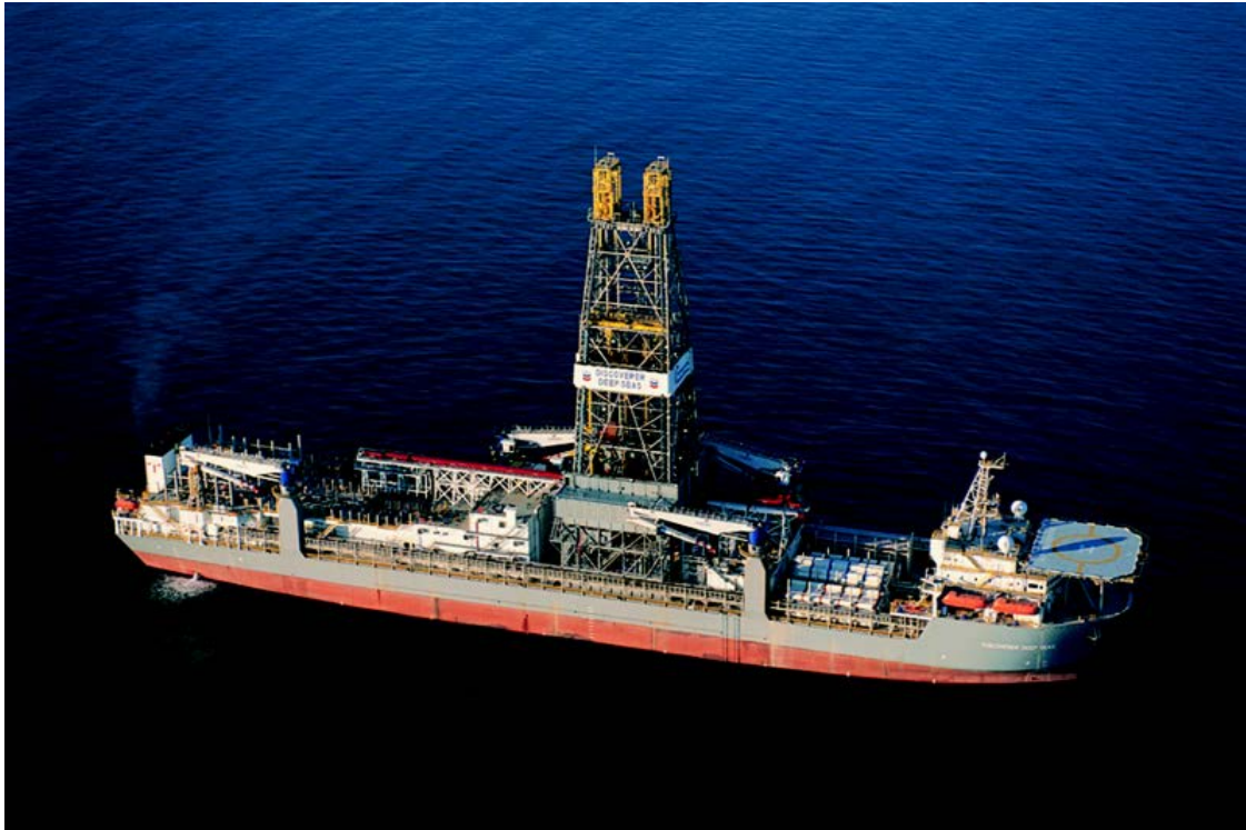
Figure 29: Ultradeepwater drill ship Transocean Discover class Discover Deep Seas. There are three of these type of units, which are 254.5 m long with a power rating of 52,000 hp and displacement of 92,800 t. Note the dual crown block for dual activity. Courtesy Transocean.
