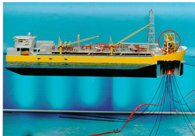
Single Point Mooring
