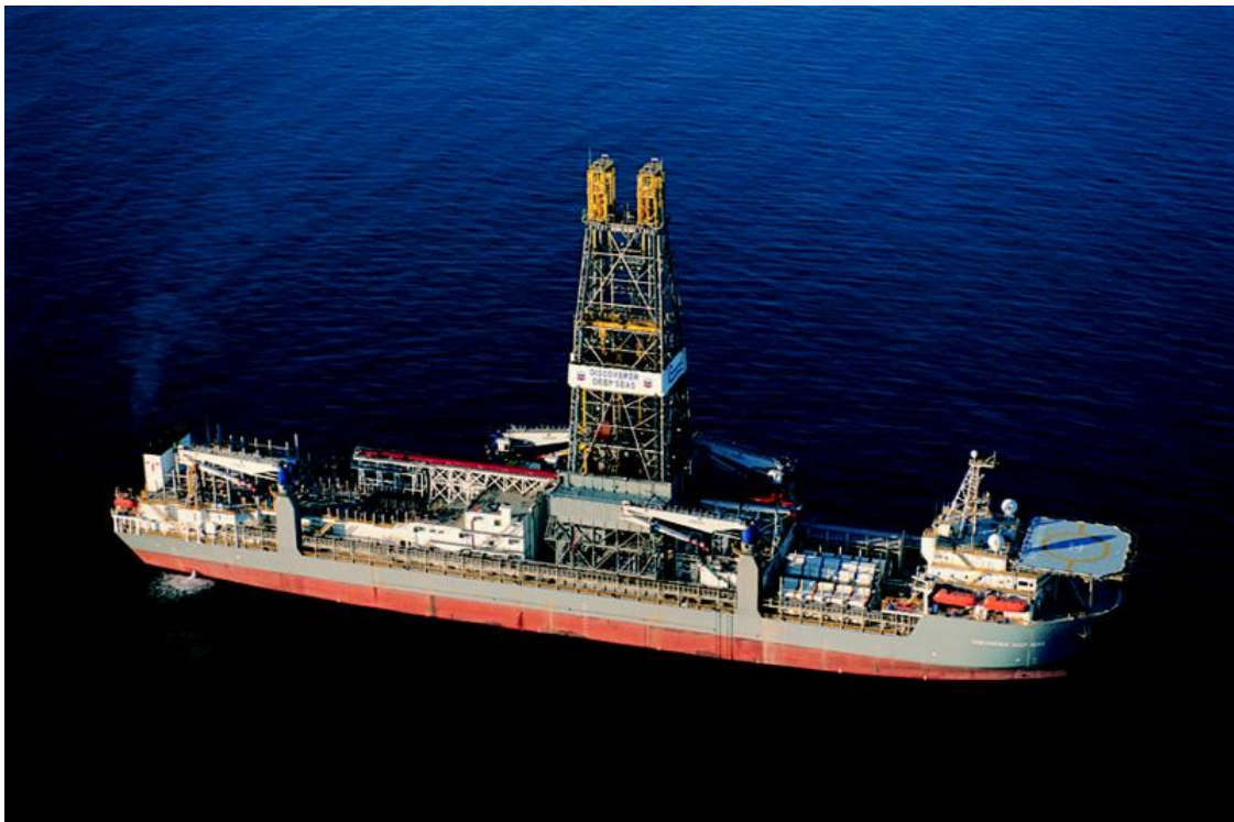
Figure 29: Ultradeepwater drill ship Transocean Discover class Discover Deep Seas. There are three of these types of units, which are 254.5 m long with a power rating of 52,000 hp and displacement of 92,800 t. Note the dual crown block for dual activity. Courtesy Transocean.
