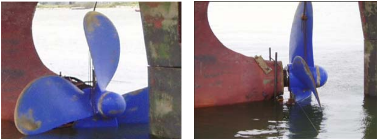
Figure 14. Face and back view of the benchmark tanker propeller painted by IS700 FR coating after 37 months in service without any cleaning
