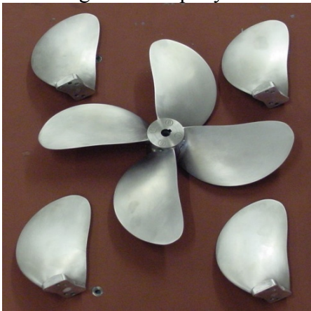
Figure 6. Model Propeller with uncoated (left) and coated (right) blades, Mutton et al (2005)
