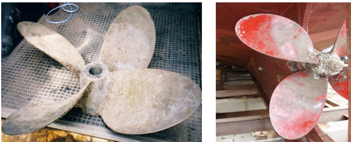
Figure 15. R/V Bernicia propeller uncoated after 14 months in service (left); coated by IS700 after 36 months in service without cleaning (right)
