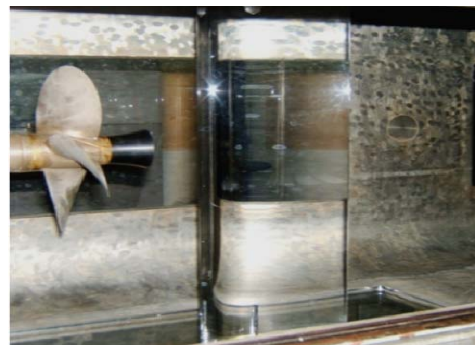
Figure 35 Use of Perspex made objects to avoid light reflection (Felli et al. , 2010)
