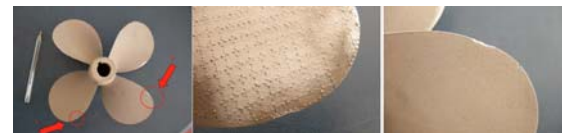
Figure 23 Propeller in Sintered Metal powder (some machining imperfections are shown) (Bazzi and Benedetti 2009)
