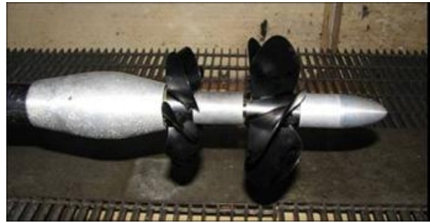
Figure 4 Open water test arrangement performed for hybrid CRP (Black and Cusanelli 2009)
