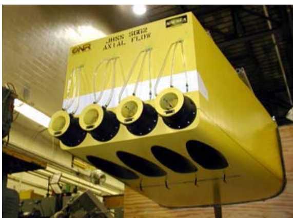
Figure 15 Four axial flow waterjet propulsion arrangement (Jessup, et al. 2008)
