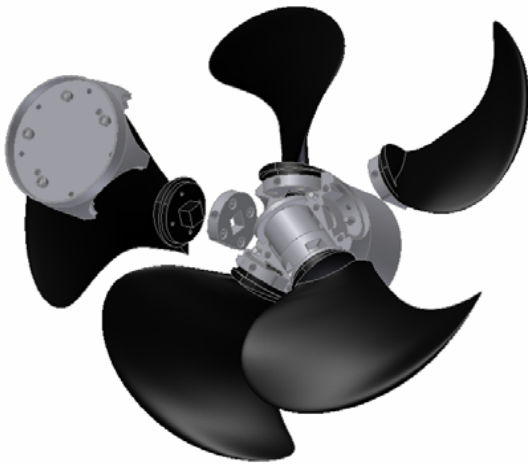
Figure 29 Exploded view of propeller hub (Jessup, et al. 2009)
