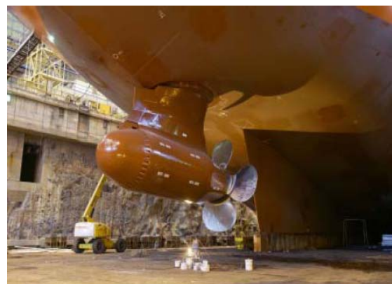
Figure 59 Lay-out of 13 MW arctic Azipod unit installed in MV "Norilskiy Nickel" (Hänninen, et al. 2007)
