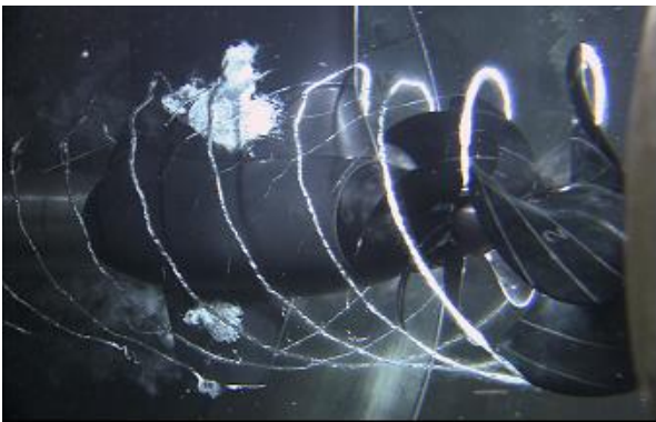
Figure 5 Cavitation testing of a hybrid CRP in the NSWCCD 36'' water tunnel (Black and Cusanelli 2009)
