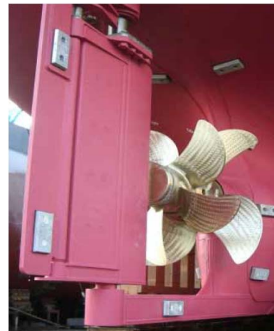
Figure 13 IHI contrarotating propellers on a chemical tanker (Inukai, 2010)
