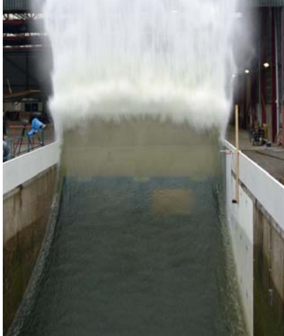
Figure 2.5.3: Full Scale Impact Tests on NO96 Elements in the Delta Flume (Kaminski & Bogaert, 2009)
