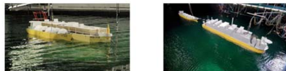
Figure 2.3.1: Examples of Side-by-side and Tandem LNG Offloading
