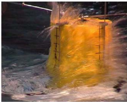
Figure 2.5.8: Wave Run-up Around a GBS (Danmeier et al., 2008)
