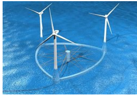
Figure 2.4.2: Semi-sub Type Floating Wind Turbine (Phuc & Ishihara, 2009)
