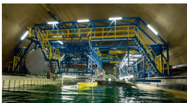
Figure 6. New wavemakers and sub carriages at MARIN depressurized basin
