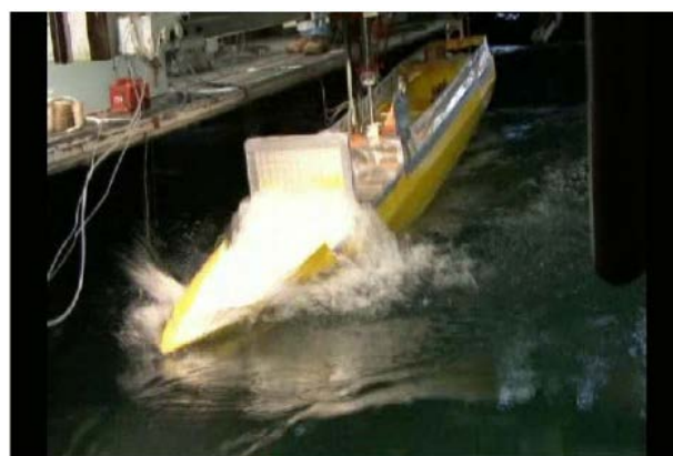
Figure 13. Model test of water on deck and slamming
