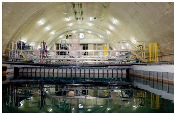
Figure 7. New wavemakers at junction of short and long walls of depressurized basin
