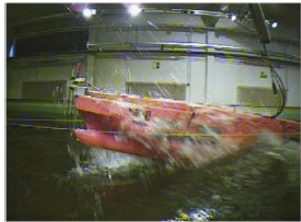
Figure 11. Model test of a Ro/Ro vessel in an extreme wave
