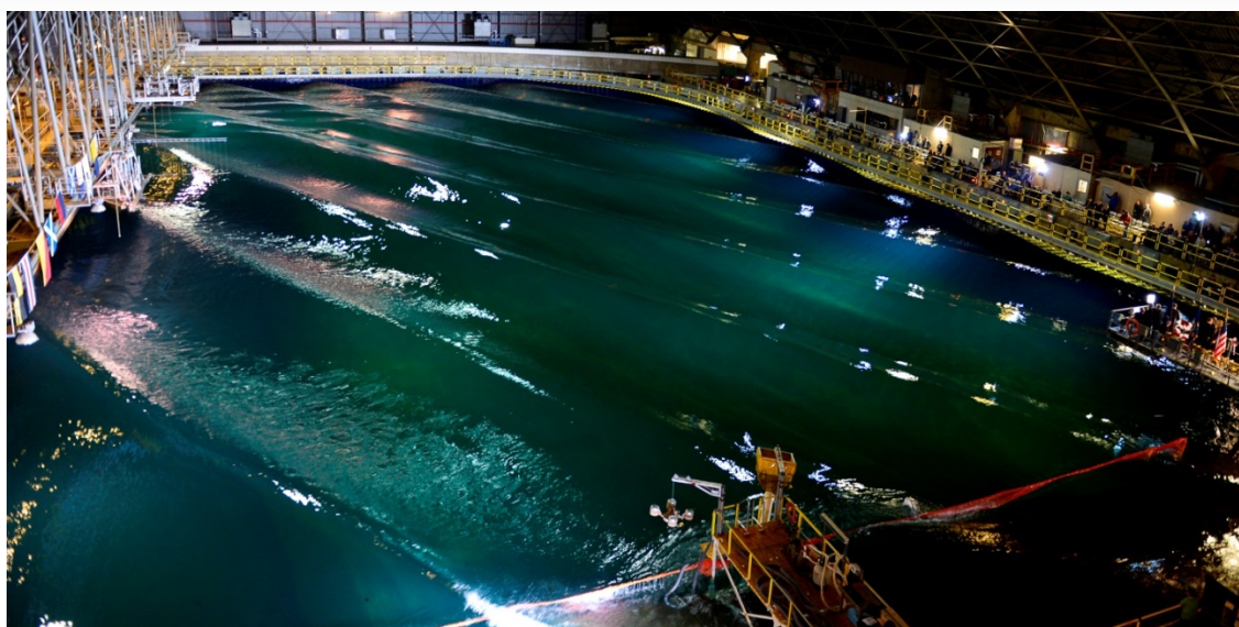
Figure 4. New Wavemaking Facility in Maneuvering and Seakeeping Basin (MASK), CDNSWC
