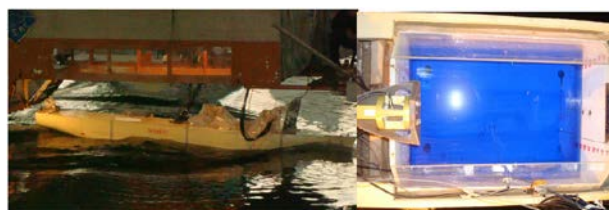
Figure 15. Model test of LNG carrier with liquid tank
