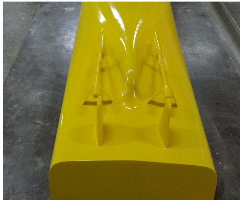
Figure 39. Installed shaft, barrel, strut and stern tube systems on a model in ITU Ata Nutku Ship Model Basin, Istanbul, Turkey.
